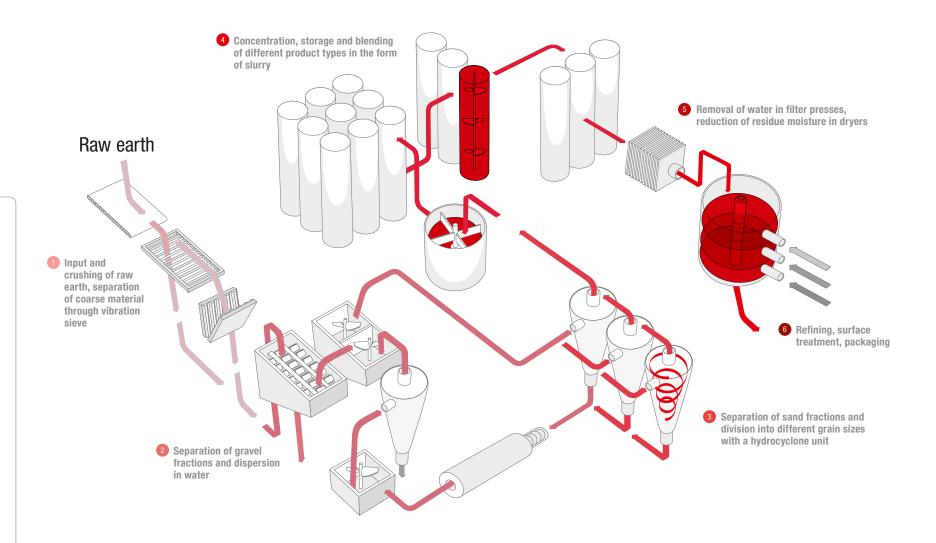
Basically speaking, our entire production process is a process of separation – only about 30% of the raw earth extracted is a usable fine product.
