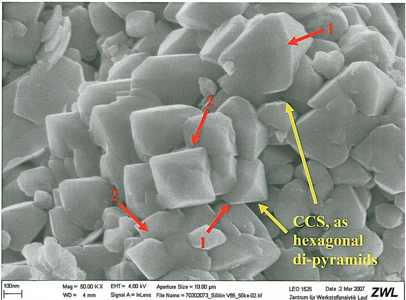
SEM – image of Sillitin V85 dated on 2<sup>nd</sup> Mar 2007. The single crypto - crystallites (CCS) of the pseudomorphosis of the High- (beta-)  $\text{SiO}_2$  - modification are not isolated. They are all affixed and stuck together by an amorphous - like  $\text{SiO}_2$  containing matrix, coated opal - like with the amorphous - like  $\text{SiO}_2$  containing matrix. The faces of the hexagonal di-pyramids may be shortened significantly (1) or are left totally (2).
