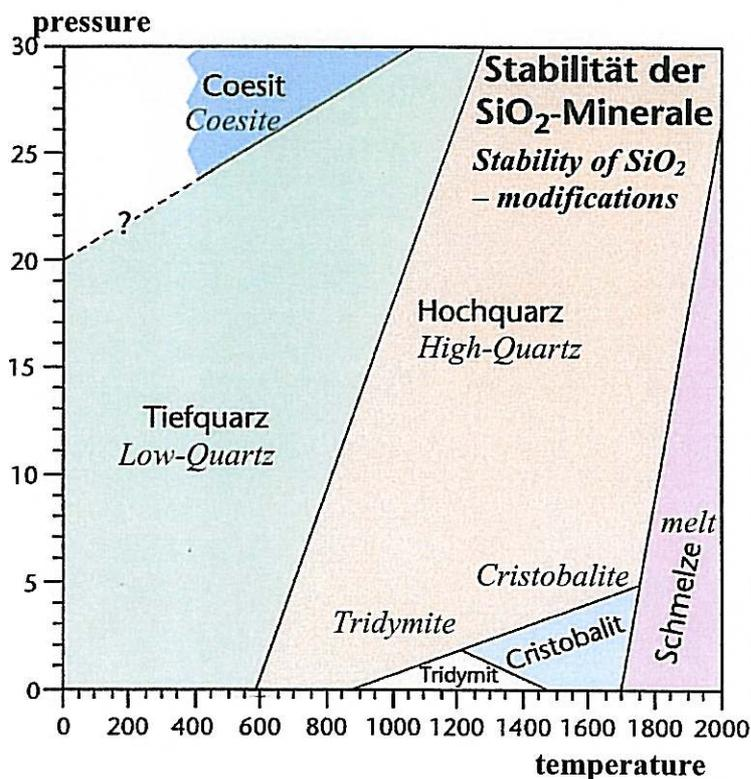
At ambient pressure the following modifications exist according to RÖSLER (1991):
