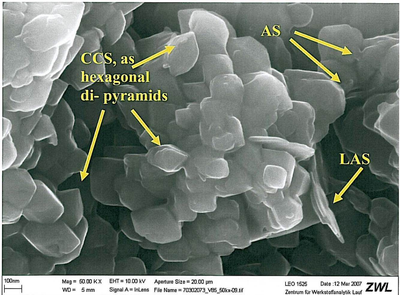
SEM – image of Sillitin V85 – quarter sample I / 2007, image acquired on 12<sup>th</sup> Mar 2007. Besides crypto - crystalline (CCS) and amorphous (AS) SiO<sub>2</sub> – phases there are visible lamellar Alumo-Silicates (LAS). No isolated SiO<sub>2</sub> – crystallites could be identified; all of them are affixed and stuck together by an amorphous – like SiO<sub>2</sub> containing matrix, coated opal – like with the amorphous – like SiO<sub>2</sub> containing matrix.
