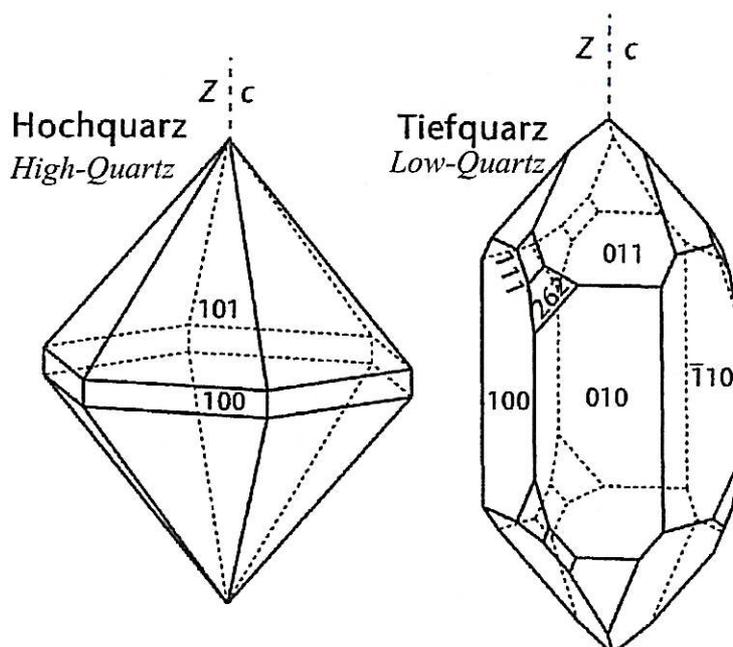
As native Low-Quartz appears as well formed crystallites in different shapes, the crystallites of naturally formed High-Quartz mostly develop hexagonal di-pyramids. The faces of the hexagonal di-pyramids may be shortened significantly or are left totally.
