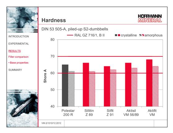
Hardness was determined on three piled-up S2-dumbells.
