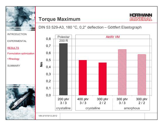
In general, the torque maximum goes down with an increased filler and oil loading, quite as should be expected in view of the decreased polymer content. The same trend, and stronger than for the increased filler loading, is true for the reduced peroxide dosing, as confirmed by the comparison of 300 phr Aktifit VM with the 2 / 2 blend vs. 400 phr Aktifit VM with the 3 / 3 peroxide blend in the crystalline EPDM grade.
