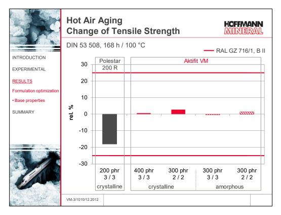
All compounds loaded with Aktifit VM during hot air aging give  $\pm 0$  % changes in tensile strength, whereas the reference compound comes out with a double-digit negative result.
