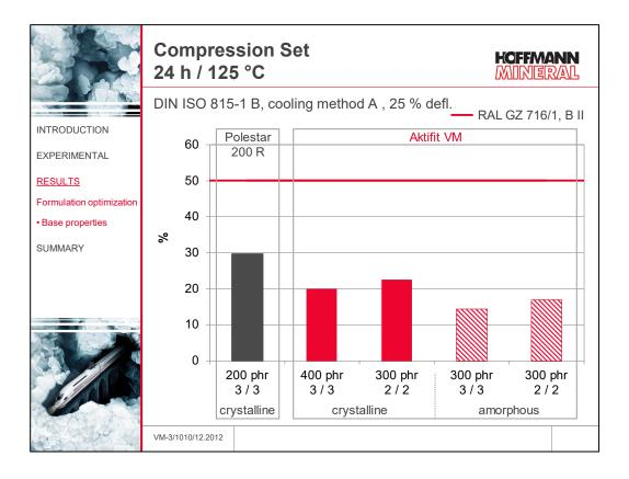
The determination of the compression set was run under the more stringent conditions at 125 °C, and the results in the graph are compared with the requirements of the RAL GZ 716/1, B II for 22 hours at 70 °C. It is very evident that even at the higher test temperature results largely below 50 % can be obtained. This means, the principal function "sealing over long periods of time" has been further improved.
