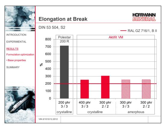
The results for the elongation at break of the compounds loaded with Aktifit VM, as a result of the surface treatment of the filler, are lower than for the control which contains the non-treated calcined clay Polestar 200 R. All compound variations with Aktifit VM surpass the minimum value of 200 % as specified in the standard.
