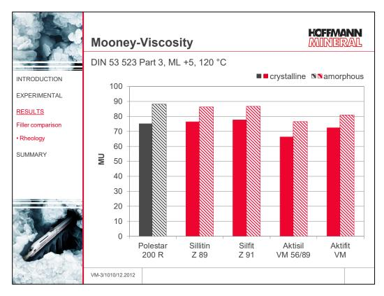
The graph shows that the results for the non-treated fillers come out at a comparable level. The viscosity with Aktifit VM is somewhat lower, and the lowest results are obtained with Aktisil VM 56/89.
