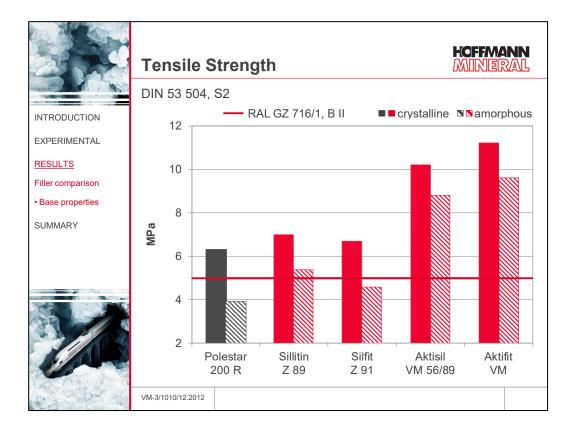
The crystalline EPDM allows to comply with the tensile strength specified in RAL GZ 716/1, B II with all fillers tested. The non-treated grades Polestar 200 R, Sillitin Z 89 and Silfit Z 91 are found at a similar level. The surface treatment of Aktisil VM 56/89 and Aktifit VM leads to a marked increase of the tensile strength for both fillers.
