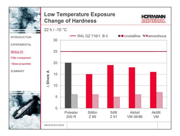
The biggest change in hardness after 22 hours of exposure to -10  $^{\circ}$ C is registered with the crystalline EPDM loaded with Polestar 200 R. Silfit Z 91 and Aktisil VM 56/89 come off slightly lower. Sillitin Z 89 and Aktifit VM in the crystalline elastomer show comparably the lowest hardness changes.
