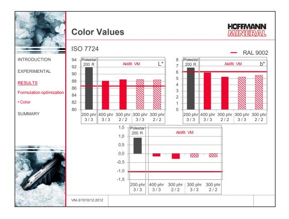
In spite of the loading level increased to 400 phr, Aktifit VM is capable to obtain the b\* value as required for the grey-white color of RAL 9002. At the same time, the brightness, indicated by the L\* result, comes very close to the specification requirement, and a\* remains in the negative region, as also specified in RAL 9002.
