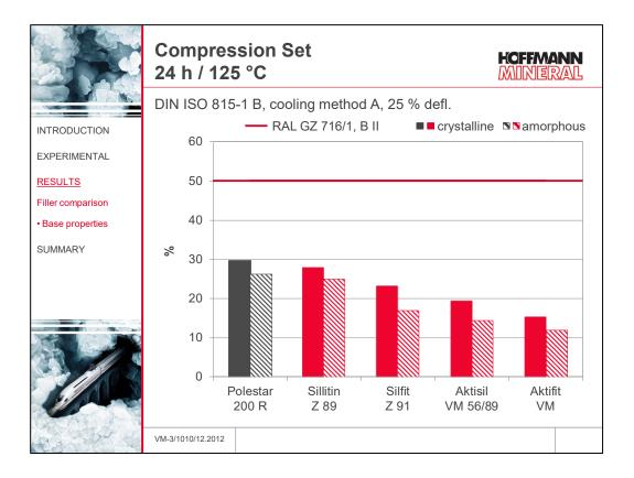
The compression set was determined under the more critical condition of 125 °C, and here it is compared with the requirement of RAL GZ 716/1, B II for 22 hours at 70 °C. Quite obviously, results largely below 50 % are obtained even at the markedly higher test temperature. This means, the major function of "sealing over long periods of time" will be further improved.
