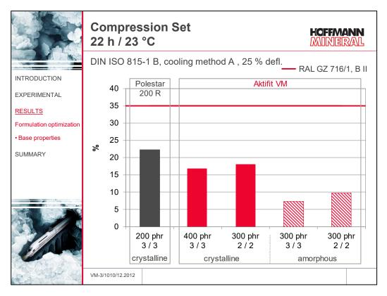
Likewise, all compounds are able to satisfy the specification at the deflection temperature of 23 °C. The results at lower level are widely comparable with what has been found at 125 °C. However, here marked difference becomes evident between the crystalline and the amorphous EPDM grades. When using the 3 / 3 peroxide blend in the amorphous polymer with a loading of 300 phr Aktifit VM, a compression set of distinctly below 10 % can be realized.
