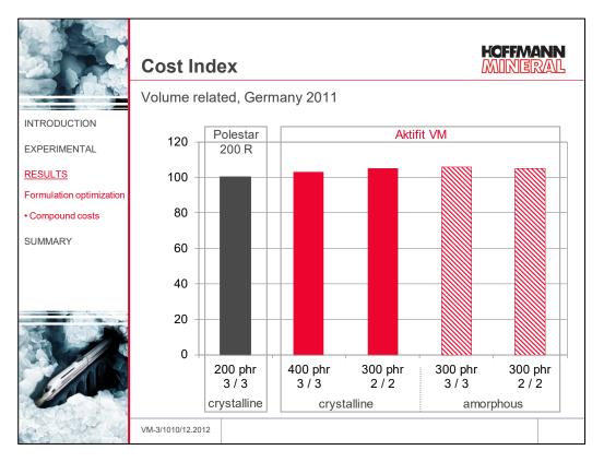
The plot clearly shows that in spite of the higher price of the Aktifit VM, the costs of the individual compound variations change only to a marginal extent. The compounds with 300 phr Aktifit VM come out around an increase of 5 %, and the higher loading of 400 phr allows even to cut that figure in half.
