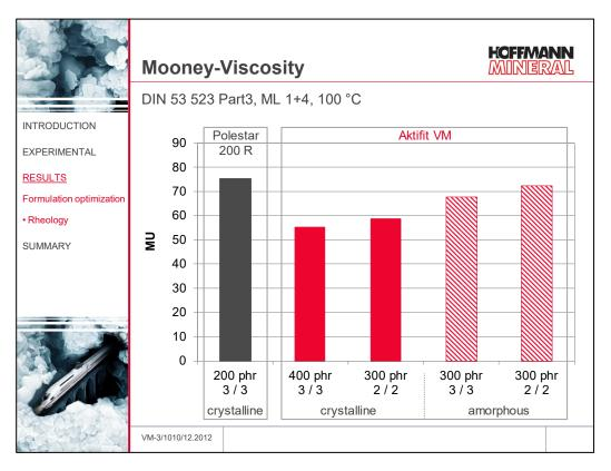
The Mooney viscosities of the two Aktifit VM compounds in the amorphous EPDM come out at a comparable level somewhat below the reference compound. With the crystalline grade, the viscosities with Aktifit VM are still somewhat lower.
