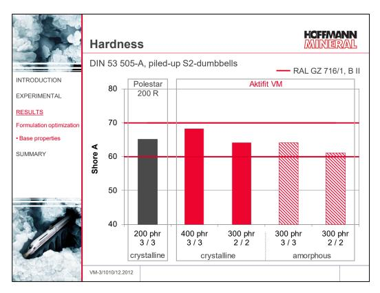
Hardness was determined on three piled-up S2-dumbbells.
