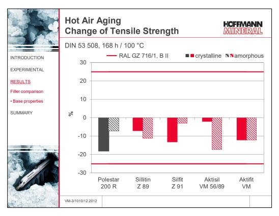
Likewise, between the changes of the tensile strength after hot air aging no big difference can be observed between the the fillers respectively the elastomer grades. The requirements of the standard are satisfied without problems in all cases.
