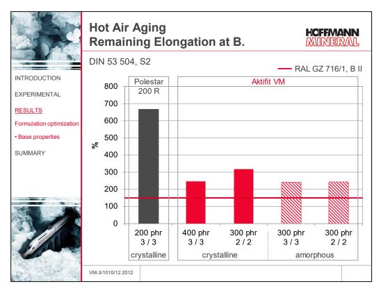
Also after hot air aging all compounds loaded with Aktifit VM reach the elongation at break specified in the pertinent standard. The overall picture is very similar to the situation prior to aging, almost without any change.
