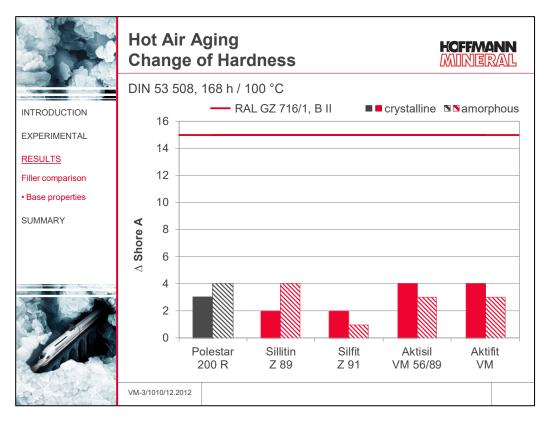
The hardness change after hot air aging 168 hours at 100 °C does not show any significant differences neither between the individual fillers nor between the two EPDM grades. All compounds remain largely below the maximum specified limit of the standard.
