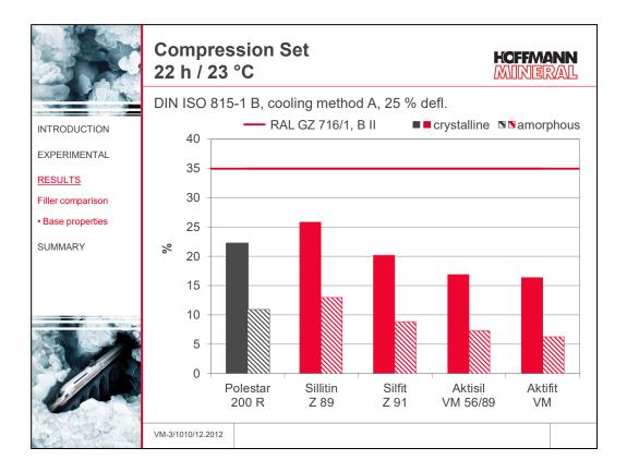
Equally, when tested 22 hours at 23 °C, the specification of the standard is satisfied with all fillers.
