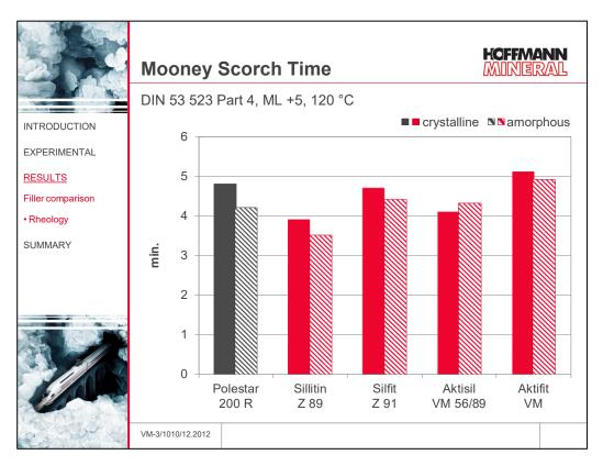
The shortest scorch time is imparted by Sillitin Z 89. The two calcined non-treated fillers Polestar 200 R and Silfit Z 91 come out somewhat longer. As a result of the surface treatment, the scorch times with Aktisil VM 56/89 and Aktifit VM are marginally longer in comparison with their base products Sillitin Z 89 and Silfit Z 91.
