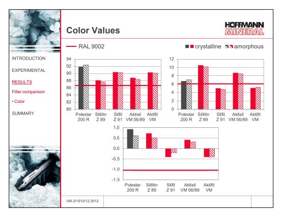
The three graphs clearly indicate that Polestar 200 R allows to come very close to the  $b^*$  requirement of the RAL 9002 specification, but this with a too high brightness (as shown by the L\* value), and instead of a required greenish, a reddish tint is evident, as confirmed by the positve a\* result.
