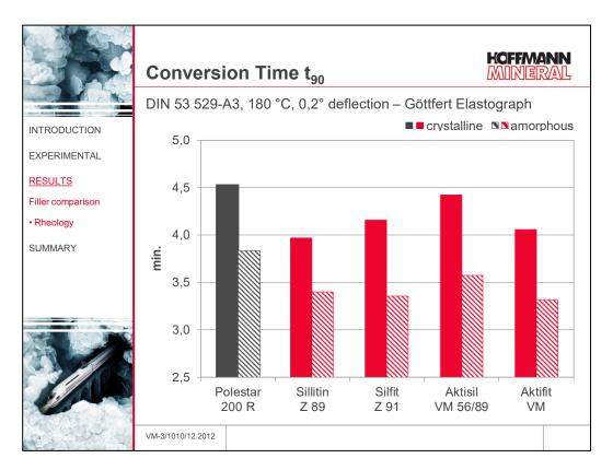
The conversion time  $t_{90}$  with Aktisil VM 56/89 is similar to the result with Polestar 200 R. Sillitin Z 89, Silfit Z 91 and Aktifit VM give somewhat shorter conversion times, which all are found at a comparable level. This shorter time requirement should represent a favour-
