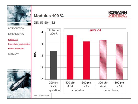
All compounds loaded with Aktifit VM surpass the 100 % modulus of the reference compound despite the higher filler and oil loading and the reduced peroxide concentration. The highest modulus is obtained with 400 phr Aktifit VM in combination with the 3 / 3 peroxide blend in the crystalline EPDM elastomer.
