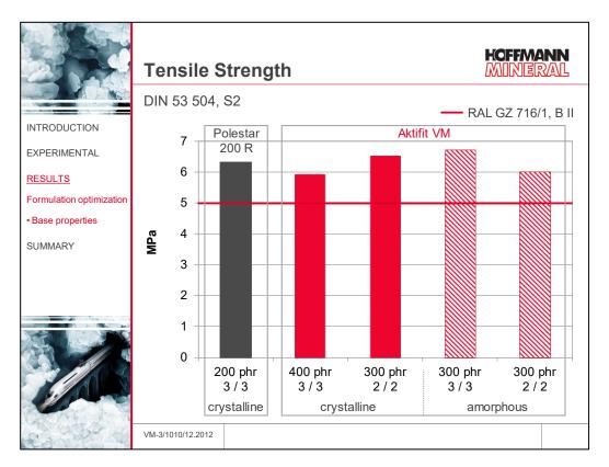
All compounds come out with a tensile strength comparable with the lowly loaded reference with Polestar 200 R, and all meet the level specified in RAL GZ 716/1, B II.
