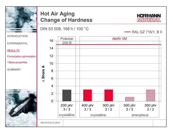
With regard to hardness changes after hot air aging, no significant difference can be observed between the individual compound variations. All compounds are able to satisfy the requirement of the standard without problems.
