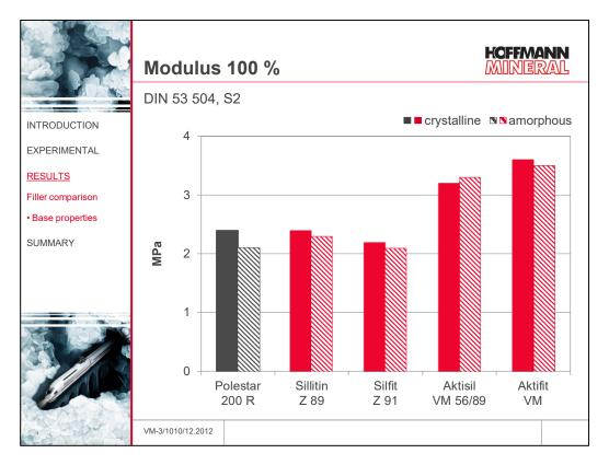
The modulus results at 100 % elongation of the non-treated fillers come out at a similar level, and this below those of the treated grades. Aktifit VM gives the highes moduli. No significant difference is seen here between the two elastomer grades.
