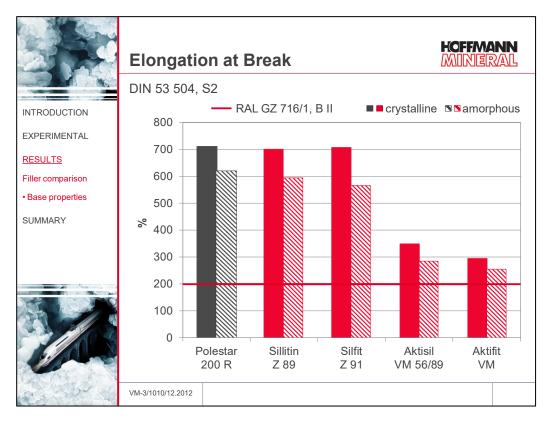
The non-treated fillers impart comparable elongations which, as expected, are higher than for the treated grades. The results with the amorphous EPDM are somewhat below those with the crystalline grade.
