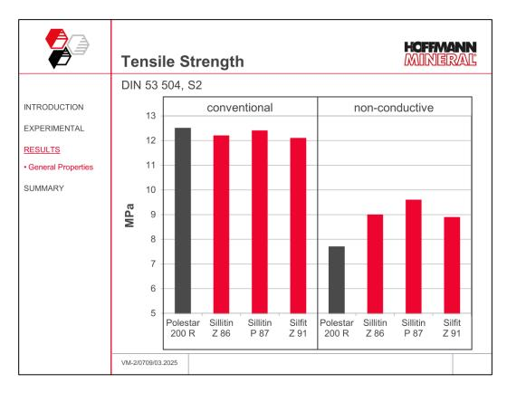
In the conventional formulations, the tensile strength does not show any significant difference between the individual fillers.
