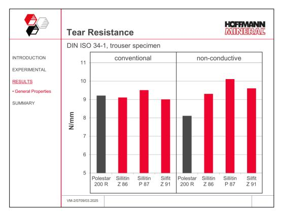
The filler selection in the conventional formulations has no significant effect on the tear resistance, as shown in the graph.
