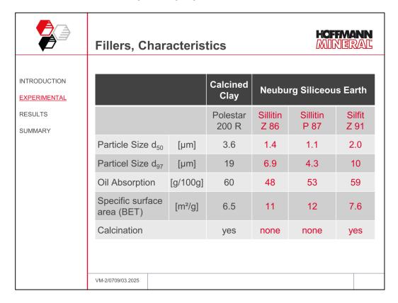
Silfit Z 91 was evaluated in comparison with two standard grades of Neuburg Siliceous Earth as well as a calcined clay.
