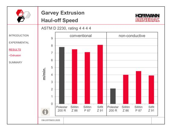
As can be seen in the graph, the conventional versions come out with marginal differences with respect to the maximum output for qualitatively good extrusions.
