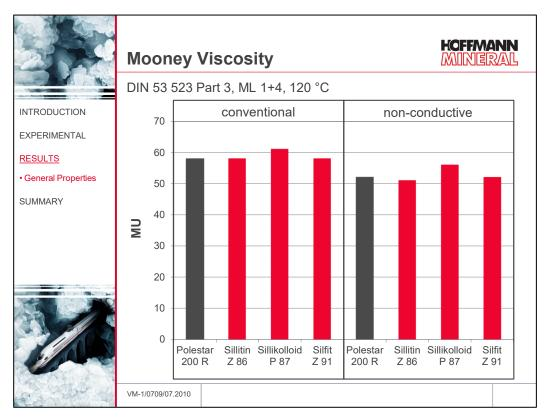
The graph indicates that Silfit Z 91 does not give any significant differences versus the standard Siliceous Earth grades and the calcined clay.
