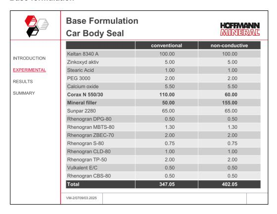
Keltan 8340 A: EPDM, amorphous Zinkoxyd aktiv: zinc oxide active Stearic Acid: processing aid
