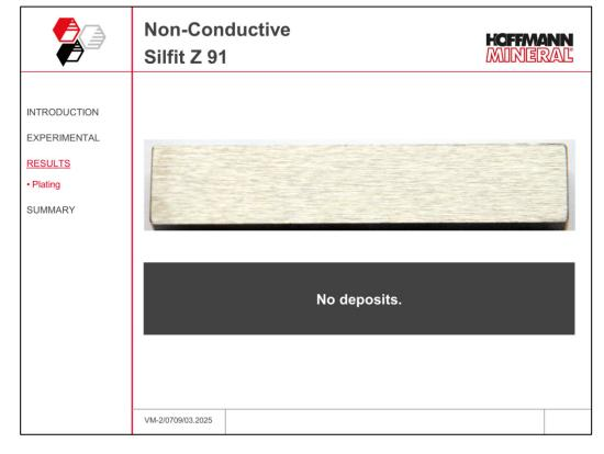
Similar to the conventional formulation, also in the non-conductive compound which contains a higher mineral filler loading, Silfit Z 91 does not give rise to any deposits. The visual observation at 100x magnification confirms this result. Filler induced deposits, therefore, can be largely or even totally avoided by working with Silfit Z 91.
