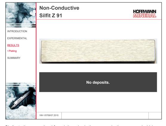
Similar to the conventional formulation, also in the non-conductive compound which contains a higher mineral filler loading, Silfit Z 91 does not give rise to any deposits. The visual observation at 100x magnification confirms this result. Filler induced deposits, therefore, can be largely or even totally avoided by working with Silfit Z 91.
