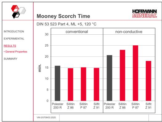
The viscosity increase from the minimum by 5 units with all fillers takes sufficiently long time. In the conventional formulation, all compounds come out with about 15 minutes. The partial replacement of carbon black increases the scorch time with the calcined clay and the standard Siliceous Earth grades considerably, with Silfit Z 91, by contrast, only moderately.
