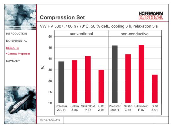
The test conditions for the compression set according to the VW test standard 3307 were 70 hours at 100  $^{\circ}$ C under 50  $^{\circ}$  deflection, cooling down for 3 hours (still under deflection), and a relaxation time of 5 seconds .
