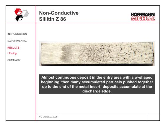
With Sillitin Z 86 in the electrically non-conductive compound, a continuous deposit is formed at the entry area with a w-shaped onset. After that, many pushed-together particle accumulations are visible up to the end of the metal insert, which gather close together at the exit edge. Deposits can be seen on the surface opposite the metal insert, too. The visual assessment at 100x magnification confirms this result.
