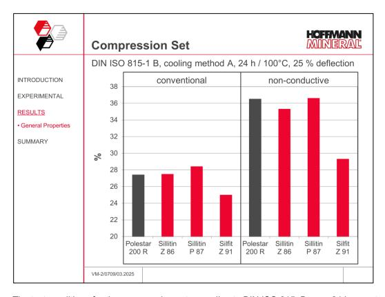
The test conditions for the compression set according to DIN ISO 815, B were 24 hours at 100 °C under 25 % deflection. The figure shows that in the conventional as well as in the non-conductive compounds the calcined clay and the standard Siliceous Earth grades impart a similar level. Silfit Z 91, by contrast, allows arriving at the lowest compression set results both in the conventional and in the non-conductive formulations.
