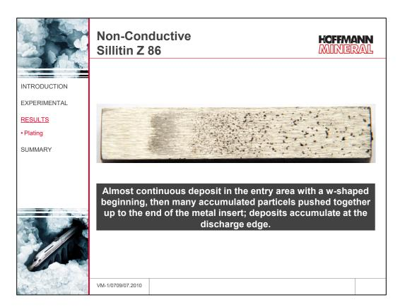
With Sillitin Z 86 in the electrically non-conductive compound, a continuous deposit is formed at the entry area with a w-shaped onset. After that, many pushed-together particle accumulations are visible up to the end of the metal insert, which gather close together at the exit edge. Deposits can be seen on the surface opposite the metal insert, too. The visual assessment at 100x magnification confirms this result. Sillikolloid P 87 shows similar characteristics.
