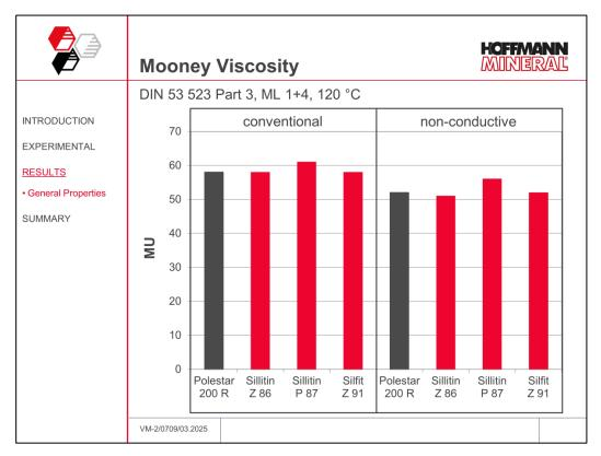
The graph indicates that Silfit Z 91 does not give any significant differences versus the standard Siliceous Earth grades and the calcined clay.
