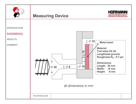
Here the dimensions of the adapted die and the measuring device are indicated.
