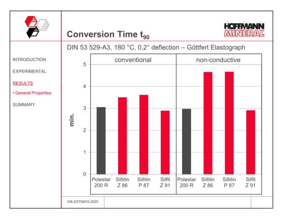
The conversion times  $t_{90}$  are fairly short for all compounds. The trend towards shorter conversion times of the calcined products comes out more pronounced in the non-conductive formulation. This way, Silfit Z 91 offers a markedly shorter  $t_{90}$  than Sillitin Z 86 or Sillitin P 87.
