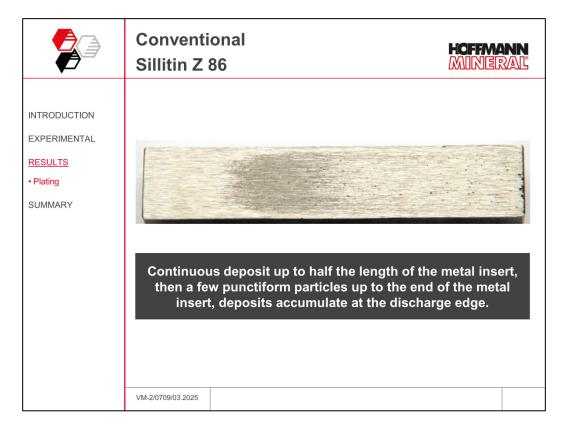
With the conventional formulation loaded with Sillitin Z 86, a continuous deposit is formed on half of the metal insert and then some punctiform particles are detected up to its end, with a certain accumulation at the exit edge. At the end of the test, deposits are also visible on the surface opposite the metal insert. The visual evaluation at 100x magnification confirms these results.
