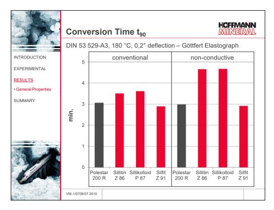
The conversion times  $t_{90}$  are fairly short for all compounds. The trend towards shorter conversion times of the calcined products comes out more pronounced in the non-conductive formulation. This way, Silfit Z 91 offers a markedly shorter  $t_{90}$  than Sillitin Z 86 or Sillikolloid P 87.
