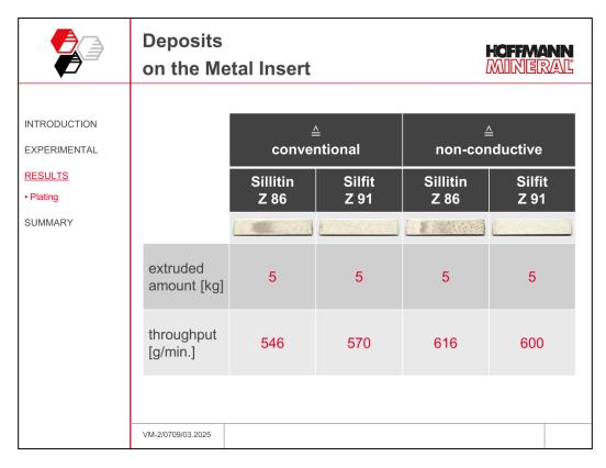
Of each compound, 5 kg were extruded, after which the metal inserts were removed and visually assessed.
