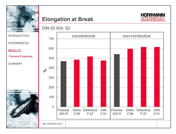
As shown in the graph, in the conventional compounds the highest elongation at break is obtained with Sillikolloid P 87; Silfit Z 91, Sillitin Z 86 and the calcined clay come out at a somewhat lower level.
