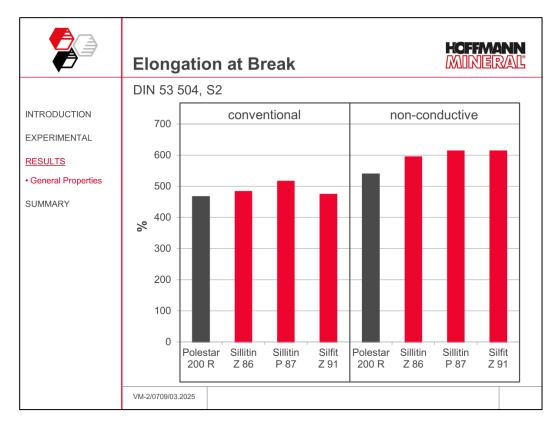
As shown in the graph, in the conventional compounds the highest elongation at break is obtained with Sillitin P 87; Silfit Z 91, Sillitin Z 86 and the calcined clay come out at a somewhat lower level.
