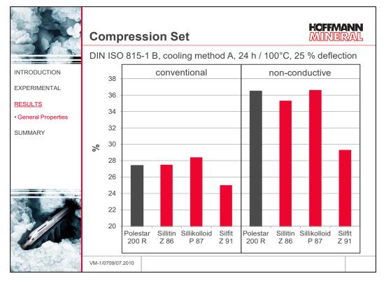
The test conditions for the compression set according to DIN ISO 815, B were 24 hours at 100 °C under 25 % deflection. The figure shows that in the conventional as well as in the non-conductive compounds the calcined clay and the standard Siliceous Earth grades impart a similar level. Silfit Z 91, by contrast, allows arriving at the lowest compression set results both in the conventional and in the non-conductive formulations.
