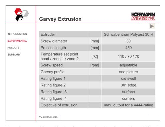
For each compound, it was tried to arrive at a maximum length output for a "4444" rating (4 is the best rating in the Garvey test, so 4444 confirms very good swelling, 30° edge, surface quality and corner shaping).
