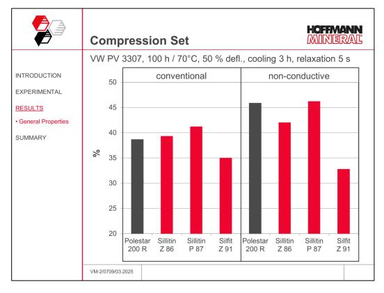
The test conditions for the compression set according to the VW test standard 3307 were 70 hours at 100  $^{\circ}$ C under 50  $^{\circ}$  deflection, cooling down for 3 hours (still under deflection), and a relaxation time of 5 seconds .
