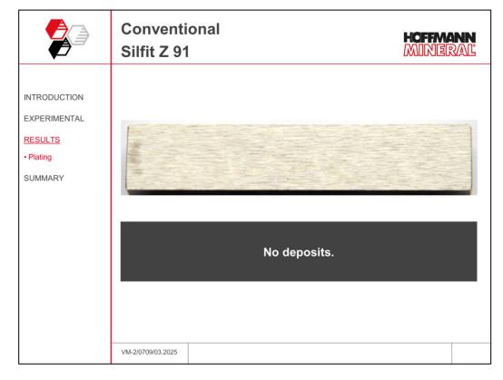
As evident from the figure, with Silfit Z 91 no deposits can be spotted on the metal insert. The visual evaluation at 100x magnification confirms this result.
