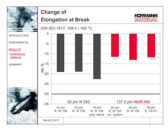
Likewise, the elongation at break of the compounds with Aktifit AM during oil immersion go down less than with the carbon black mixes which is why their absolute figures manage to level up a bit, as shown in the lower graph.
