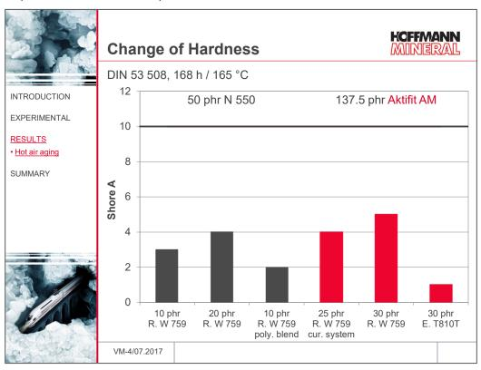
The change of hardness after hot air aging of the carbon black loaded compounds comes out similar to the Aktifit AM mixes, with both meeting the PSA specification without any problems.
