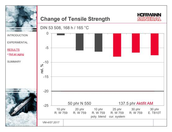
The tensile strength as well as the elongation at break (lower graph) of the carbon black loaded or equally the Aktifit AM containing compounds do not significantly react to aging in hot air.
