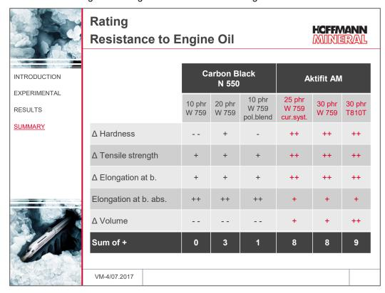
When comparing the individual parameters concerning oil resistance, however, the benefits of Aktifit AM come out clearly. Here too the absolute figures for the elongation at break are lower than for the carbon black but the requirements with respect to decrease of hardness and volume change cannot be met neither with an increased plasticizer addition nor by blending Vamac Ultra IP with Vamac VMX-3110.
