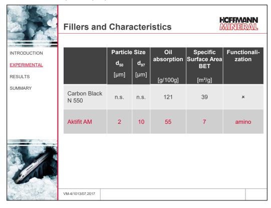
The low figures for the oil absorption and the specific surface area indicate that the product Aktifit AM, modified with an amino functional group, compared with carbon black N 550, is a filler of rather low activity.
