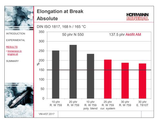
Overall, the oil resistance tests of the compounds reveal a clear advantage for the use of Aktifit AM in place of carbon black. In particular, the critical parameters volume increase and hardness decrease can be positively influenced with Aktifit AM.
