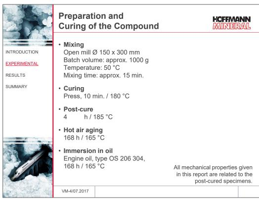
The compounding was done on a laboratory mill (Schwabenthan Polymix 150 L), with the rubber added at 50 °C, milled and pulled out to a uniform sheet. Subsequently, the filler
