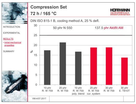
The higher Rhenosin W 759 addition leads to an increase of the compression set in the carbon black compounds, whereas no change in the results can be observed in the compounds based on the blend of Vamac Ultra IP and Vamac VMX-3110.
