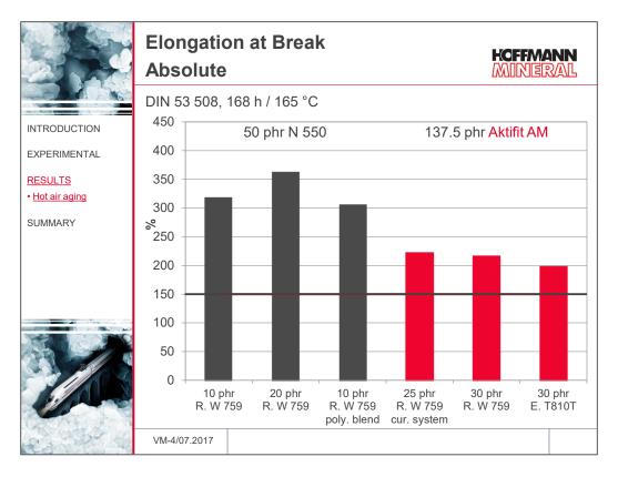
Elongation at break only is subject to minimal changes which means the results largely remain at the initial level.
