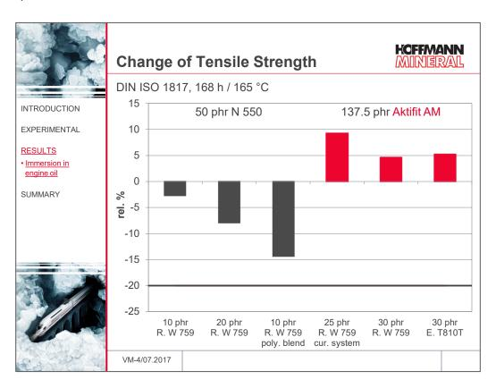
It is true that the change of tensile strength for all compounds results relatively low, but still a marked trend towards generally higher figures is evident for the compounds loaded with Aktifit AM while the tensile strength of the carbon black loaded rubbers rather points to a lower level.
