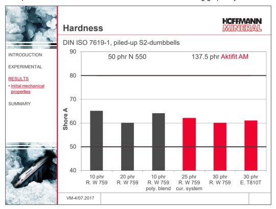
The high loading of Aktifit AM in combination with the increased plasticizer content leads to hardness values on a comparable level with the carbon black compounds which, however, contain a lower amount of filler.
