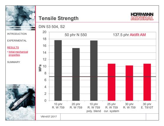
With respect to the tensile strength, the lower activity of Aktifit AM compared to the carbon black results in lower figures which, however, well meet the requirements of the PSA specification. Overall it does not make any difference if Rhenosin W 759 is replaced by Edenol T810T, or if the dosage is somewhat reduced and the crosslinking system slightly modified.
