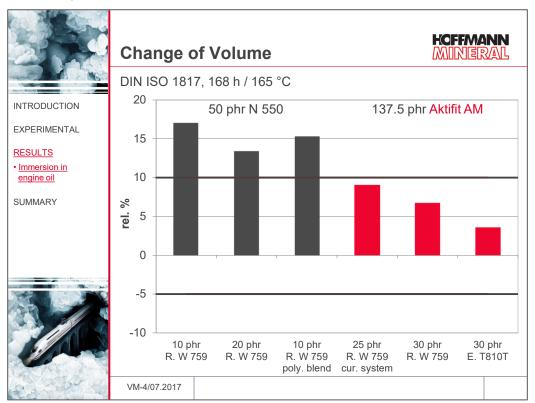
The reference compound loaded with 50 phr carbon black N 550 for the first time is not able to meet a requirement of the PSA specification. The volume change comes out too high and cannot be reduced sufficiently by increasing the plasticizer content nor by using the blend of Vamac Ultra IP with Vamac VMX-3110.
