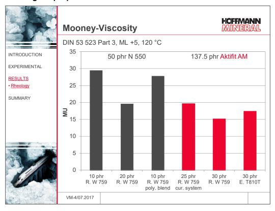
Upon increasing the plasticizer loading from 10 to 20 phr, according to expectations the Mooney viscosity will come out reduced, while blending Vamac Ultra IP with Vamac VMX-3110 practically does not affect the viscosity at all.
