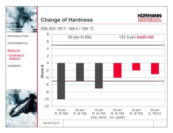
Similarly, meeting the requirement concerning the hardness change upon oil immersion is not possible with carbon black and just barely when adding 20 phr Rhenosin W 759, while all compounds loaded with Aktifit AM are able to come out within the limits of the PSA specification S 22 5106 Class 165.
