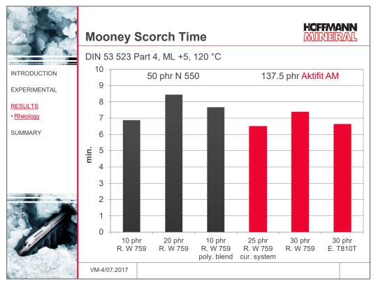
The scorch time of all of compounds comes out above 6 minutes. Basically one can say that it becomes somewhat longer with increasing plasticizer content, i.e. the result is a somewhat improved processing safety when using a high amount of plasticizer. This is also true for the blend of Vamac Ultra IP and Vamac VMX-3110. The replacement of Rhenosin W 759 with Edenol T810T does not give any significant effect.
