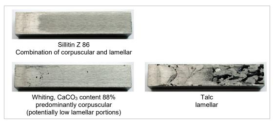
Figure 14: Comparison of fillers of different particle structure
