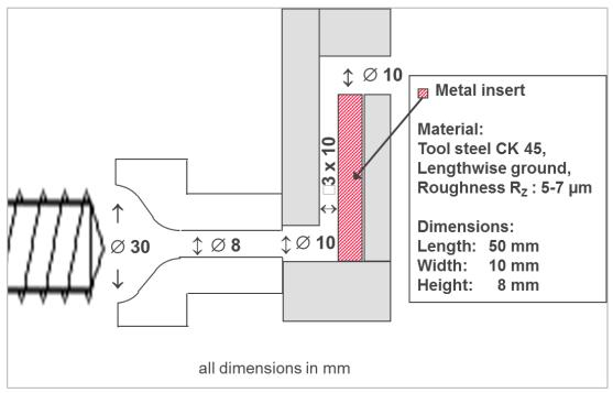
Figure 2: Schematic drawing of the front-end test device with metal insert
