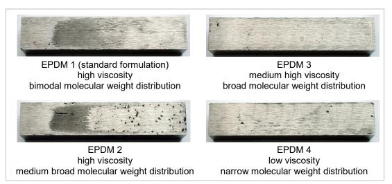
Figure 8: Metal die inserts after trials with compounds based on 4 different EPDM types
