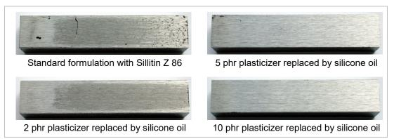
*Figure 10:* Effect of silicone oil as partial replacement of the paraffinic mineral oil plasticizer on the die-plating tendency
