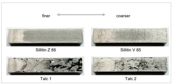
Figure 15: Effect of particle size
