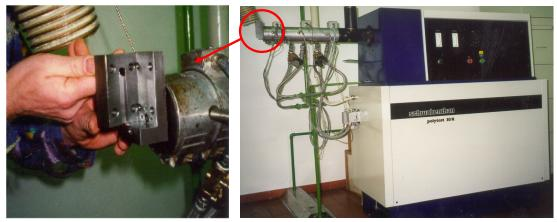
Figure 1: Special front-end test device and Schwabenthan extruder Polytest 30 R
