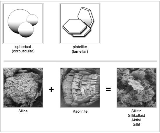
*Figure 13:* Schematic representation of various tested particle structures and SEM photographs of Neuburg Siliceous Earth
