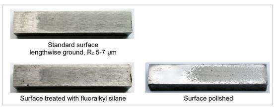
Figure 4: Effect of the die insert surface on the die-plating effect
