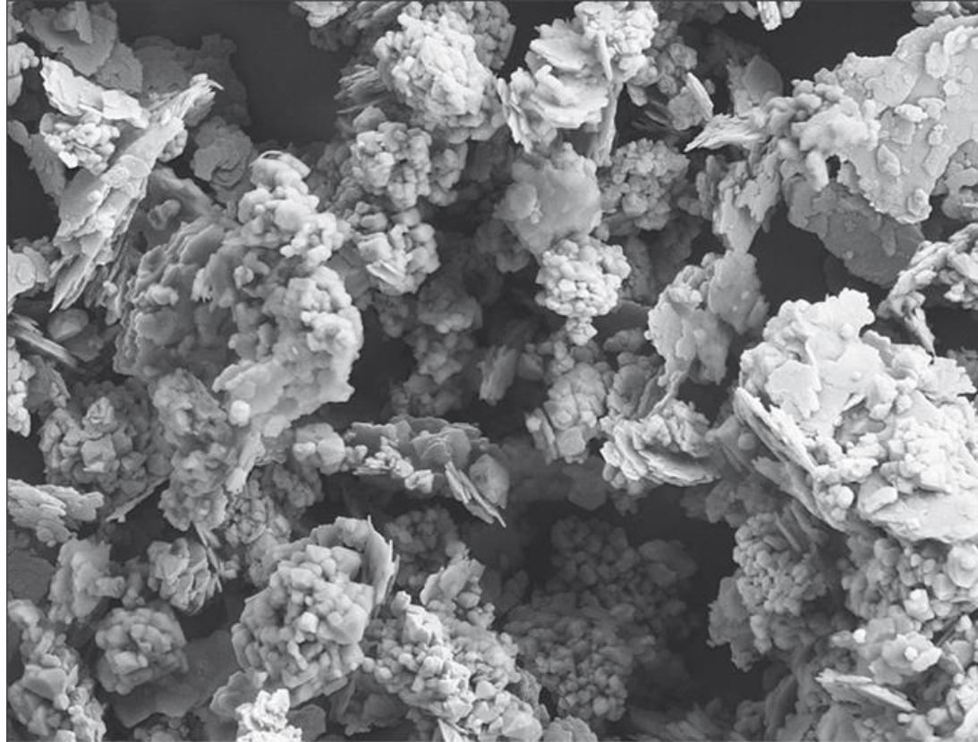
A natural combination of corpuscular Neuburg silica and lamellar kaolinite: a loose mixture impossible to separate by physical methods. The silica portion exhibits a round grain shape and consists of aggregated primary particles of about 200 nm diameter.
