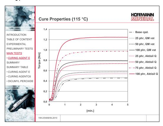
As little as 25 phr Aktisil Q almost come up to the maximum torque which will be attained with 50 phr silanized quartz flour. The graph also indicates that the torque maximum with 100 phr treated quartz flour is exceeded with 75 phr Aktisil Q.
