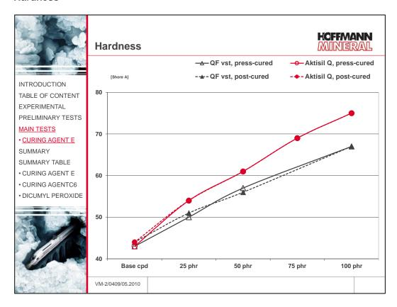
At equal loadings, Aktisil Q always leads to higher hardness than the treated quartz flour. It is clearly evident that 75 phr Aktisil Q are able to match the hardness with 100 phr of the silanized quartz flour.
