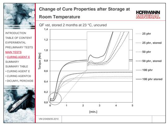
An increase of the torque minimum with 100 phr is also seen for the silanized quartz flour. In addition, there is a trend towards an increased maximum torque.
