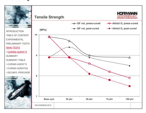
Higher filler loadings give rise to slightly reduced tensile strength. Aktisil Q at equal loadings comes out just below the silanized quartz flour. Post-cure causes an increase of tensile strength with the base compound, while the compounds with added fillers rather show a slight decrease.
