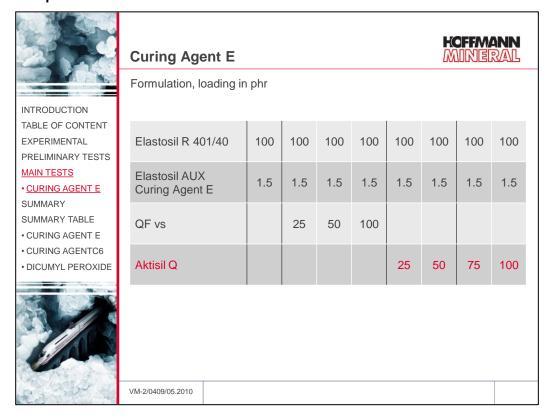
Silanized quartz flour and Aktisil Q were used at loadings of 25, 50 and 100 phr. With Aktisil Q, also a loading of 75 phr was included, because in the preliminary tests at 100 phr Aktisil Q had led to higher hardness vs. the treated quartz flour.
