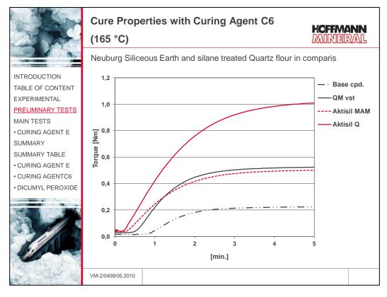
The use of Sillitin grades gives rise to unsatisfactory crosslinking, therefore these fillers will not be shown here. Aktisil MAM makes it possible to attain the torque of silanized quartz flour. Aktisil Q again shows a marked torque increase compared with the base compound or to the compound with silanized quartz flour.
