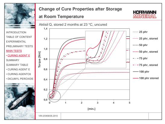
Loadings up to 75 phr Aktisil Q do not cause any significant changes in the uncured compounds. Above this loading, there is a slight decrease of the maximum torque. whereas the minimum torque increses, as shown with the 100 phr compound. In other words, a storage stability at ambient temperature (23 °C) is assured up to loadings of 75 phr.
