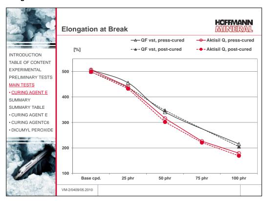
Addition of fillers causes the elongation at break to fall off, and this all the more the higher the filler loading. The graph shows that the elongation decrease is somewhat more pronounced with Aktisil Q compared to the silanized quartz flour at equal loading. When comparing the 75 phr Aktisil Q compound with the 100 phr quartz flour compound (equal hardness), the elongation at break is found on an equal level. A post-cure does not have any effects on the elongation.
