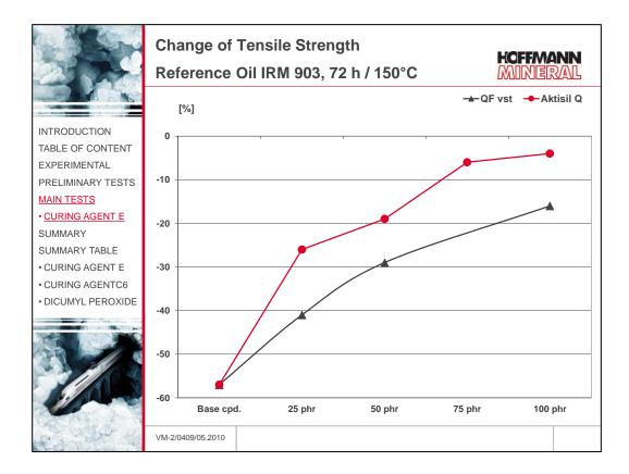
Upon immersion in Reference Oil IRM 903, the tensile strength of the base compound drops off considerably. The addition of further fillers is able to markedly reduce this effect.
