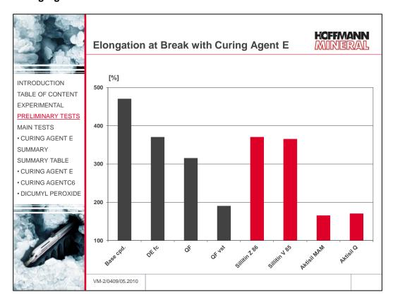
The initial elongation at break of the base compound is reduced by all fillers added. The flux-calcined diatomaceous earth, Sillitin Z 86 and Sillitin V 85 come out closest to those levels, followed by the untreated quartz flour. A surface treatment of the fillers, in HTV silicone rubber like in most other elastomers, leads to a reduced elongation at break, as confirmed by the figures for quartz flour, Aktisil MAM and Aktisil Q.
