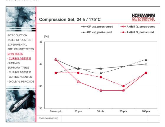
Prior to post-cure, the silanized quartz flour compound gives a compression set lower than the base compound without additional fillers prior to post-cure. However, the low level of the post-cured base compound will not be matched, even with post-cure. In total, post-curing does not show very big effects on the compression set with silanized quartz flour.
