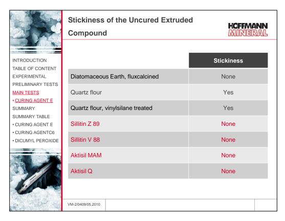
The uncured extrusions filled with quartz flour tend to exhibit a markedly higher surface stickiness, independent of a surface treatment of the filler. The diatomaceous earth and all Sillitin and Aktisil grades leave the extruded compounds free from surface stickiness.
