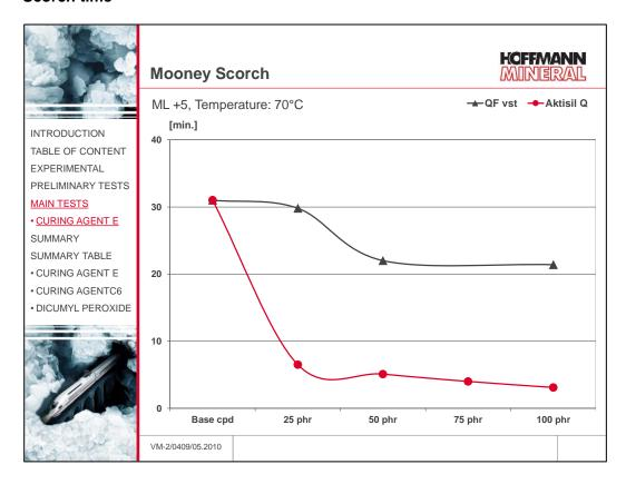
The graph shows that scorch times are becoming shorter with increasing filler addition. As already seen in the preliminary tests, this effect is highly pronounced with Aktisil Q, so here the lowest possible processing temperature should be applied. The storage stability of the compounds, however, remains ensured (see below, item "Change of curing profiles upon storage at room temperature").
