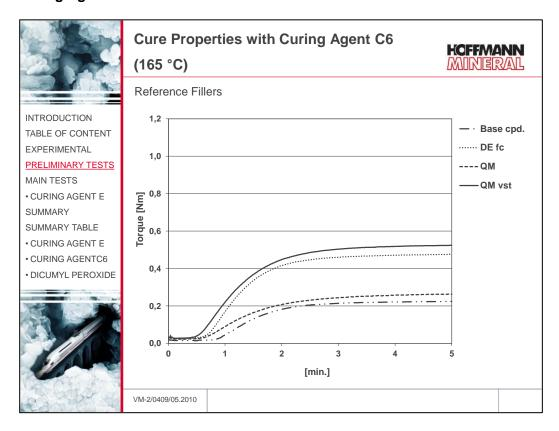
Quartz flour slightly increases the torque compared with the base compound; surface treatment brings about a marked increase. Diatomaceous earth comes out somewhat below the silanized quartz flour.
