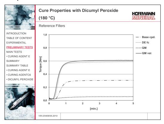
As evident from this graph, the use of untreated quartz flour with dicumyl peroxide will inhibit the crosslinking process. Quartz flour can only be used in its surface treated version. Then there is no difference in crosslinking effects with the flux-calcined diatomaceous earth, in so far as both fillers increase the torque of the base compound by a factor of two.
