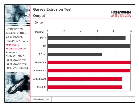
For all fillers used, the output at a screw speed of 100 rpm is found between 9 and 10 m/min, excepted the compound with silanized quartz flour, which only arrives at a much lower figure.
