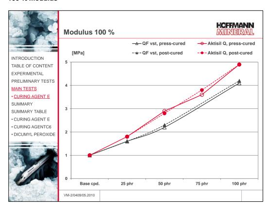
A modulus increase is more pronounced with Aktisil Q than with silanized quartz flour. Here again, hardly any influence of post-curing can be observed.
