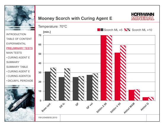
The use of diatomaceous earth and quartz flour (untreated or treated) does not give rise to significant changes in the scorch properties compared with the base compound without further added fillers. By contrast, Sillitin leads to markedly longer scorch times. With the untreated fillers such as quartz flour and Sillitin, no onset of cure can be observed. Aktisil MAM and Aktisil Q show a distinctly shortened scorch time. The individual results are given in the Appendix.
