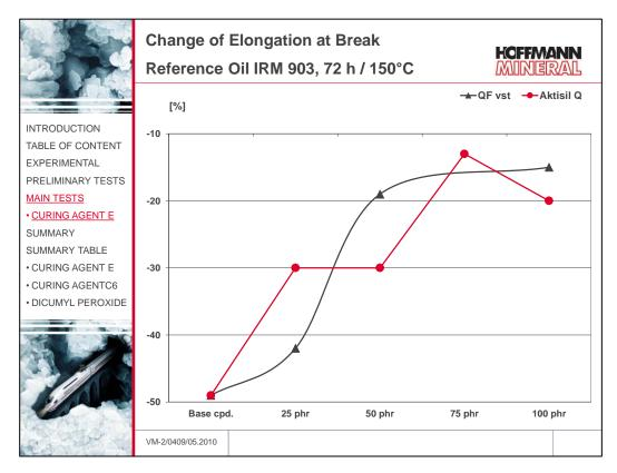
As shown in this graph, higher filler loadings tend to minimize the reducing effect on the elongation at break of the immersion in the Reference Oil. Without post-cure this statement is also valid.
