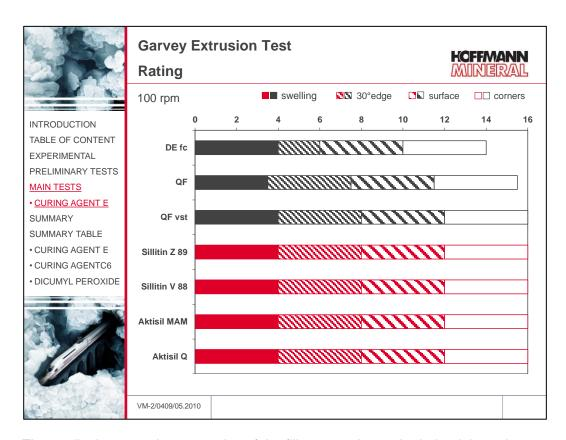
The qualitative extrusion properties of the fillers tested must be judged throughout as good. Only the flux-calcined diatomaceous earth shows a deficit in the 30° edge formation. The quality of the profile with silanized quartz flour is quite good, but as already shown in the graph above, the output is much reduced. The best results, qualitative as well as quantitative, are obtained with the Sillitin and Aktisil grades.
