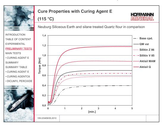
Also Sillitin V 85 and Z 86 cause a higher torque compared to the base compound without additional fillers; the level, however, remains somewhat below the silanized quartz flour. A torque increase above quartz flour is observed with Aktisil MAM, which in turn is even surpassed with Aktisil Q.
