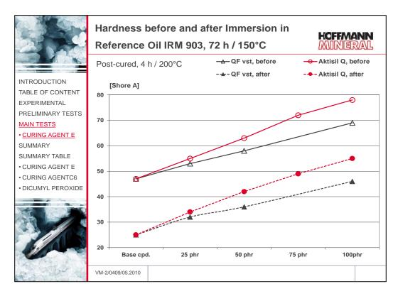
The hardness changes upon immersion in the Reference Oil are practically the same for all compounds tested. This means that the higher Shore A level with Aktisil Q is maintained also after the immersion test. This is also valid for compounds that have not been post-cured.
