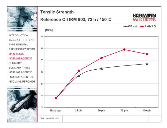
Without post-cure, the absolute values of the tensile strength with Aktisil Q are comparable to the values of the treated quartz flour.
