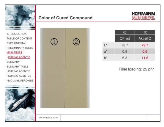
Compared with quartz flour, the compounds filled with Aktisil Q are characterized by a slight yellowish tint, identifiable by the higher b\*-value.
