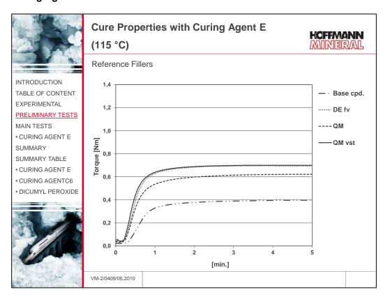
The addition of quartz flour gives rise to a marked increase of the Rheometer torque above the base compound. Surface treatment of the quartz flour leads to a further increase. Diatomaceous earth behaves similar to the treated quartz flour.
