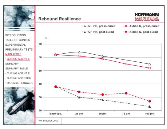
With increasing filler loadings, the rebound resilience will go down slightly. As also evident from the graph, a post-cure causes the rebound to drop off. This effect is somewhat less pronounced with Aktisil Q than with silanized quartz flour.
