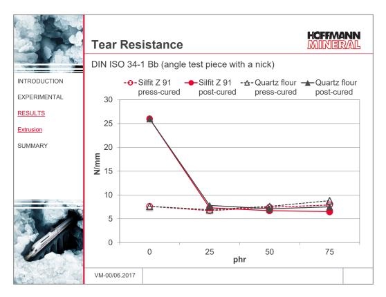
In the post-cured compounds, the addition of 25 phr filler already causes a marked drop of the tear resistance – and this irrespective of the type of filler used. With further increased loadings, no further change in the tear resistance level can be observed and there is no difference either between Silfit Z 91 and the quartz flour.
