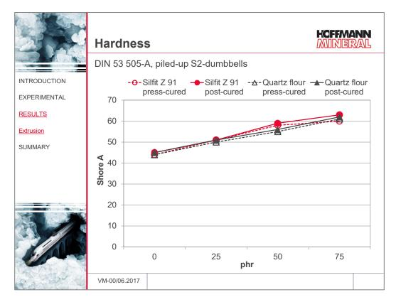
The stepwise increase of the filler loading for Silfit Z 91 and the quartz flour gives rise to comparable increases in hardness.
