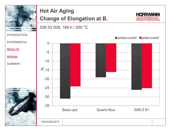
While the quartz flour addition results in a somewhat smaller change of the elongation at break during hot air aging, Silfit Z 91 remains practically on level with the base compound.
