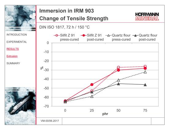
While the volume change upon immersion in reference oil IRM 903 of compounds loaded with Silfit Z 91 does not show any differences vs. those with quartz flour, with respect to changes in tensile strength they give proof of advantages. In fact, the tensile strength results of the press-cured as well as of the post-cured samples with Silfit Z 91 drop less than with quartz flour.
