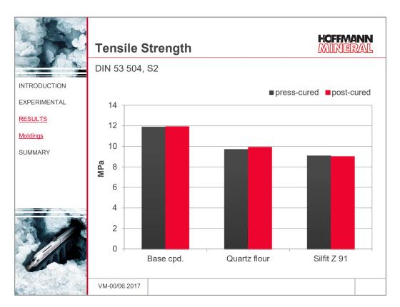
By adding the fillers, the tensile strength of the base compound is somewhat reduced. The compounds filled with Silfit Z 91 give rise to only marginally lower levels than those with quartz flour. Post-curing here shows practically no effect.
