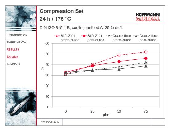
Through post-curing, the compression set of the compounds loaded with Silfit Z 91 can be decreased to a level which comes close to the quartz flour.
