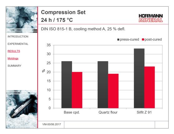
By post-curing, the compression set with Silfit Z 91 can be decreased in a way that the results arrive at a comparable level with the unfilled base compound or the quartz flour.
