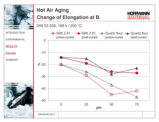
Between the two fillers, no significant differences can be found with respect to the aging in hot air (168 h / 200  $^{\circ}$ C). This is here illustrated by the changes in elongation at break. A post-cure leads to smaller changes in elongation both with Silfit Z 91 and with quartz flour.
