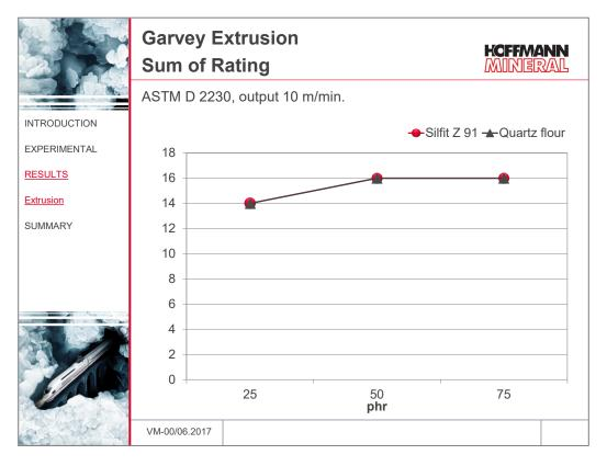
With a constant output rate of 10 m/min., no differences can be discovered between the extrudates filled with Silfit Z 91 resp. with the quartz flour.
