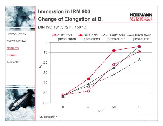
More favorable levels with the post-cured compounds containing Silfit Z 91 also result at loadings of 25 and 50 phr with respect to the elongation at break. In compounds with still higher loadings, no differences can any longer be observed between both fillers.
