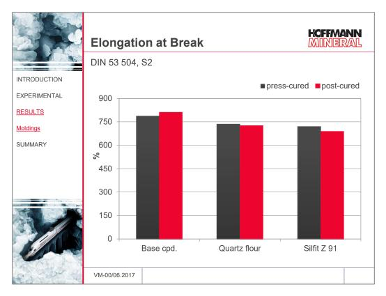
The elongation at break with 25 phr filler is only marginally lower compared with the base compound. The choice of the filler has no significant influence on the results, as little as the post-curing step.
