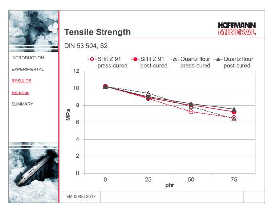
The increasing loading of fillers leads to a decline of the tensile strength of the base compound. Before post-curing, the compounds show small differences only at medium loading, while after post-cure no deviations are observed between Silfit Z 91 and the quartz flour.
