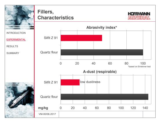
With the help of the Einlehner test which allows to assess the wear of processing machines etc., it can be confirmed that Silfit Z 91 offers a marked improvement over the quartz flour with respect to abrasivity.
