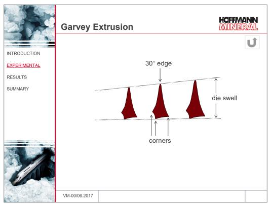
This specially developed die geometry allows to evaluate with simple means in relatively short time several compounds with respect to their extrudability and thus to obtain qualitative indications about their extrusion properties.
