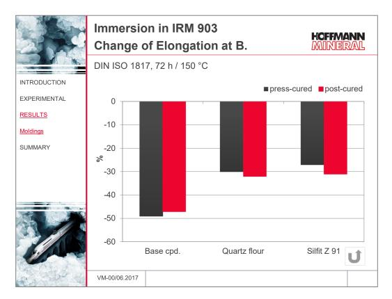
In this graph, the change of elongation at break during immersion in reference oil IRM 903 (72 h / 150  $^{\circ}$ C) demonstrates, to what extent the resistance can be improved by the addition of fillers. Silfit Z 91 and the quartz flour show comparable effects – and this before and after post-curing.
