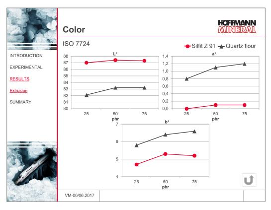
Compounds filled with Silfit Z 91 are distinctly brighter compared with quartz flour loading, as confirmed by the L\* values in the diagram. While the a\* values with Silfit Z 91 doubtless are found in the neutral region, the b\* values are clearly oriented towards a shade of blue. The result is a higher color neutrality of the compounds loaded with Silfit Z 91 in comparison with the samples with quartz flour.
