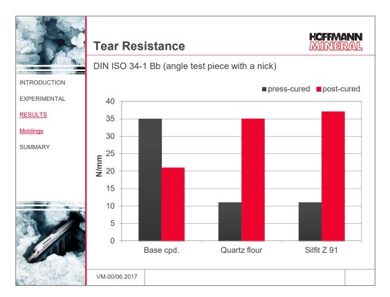
While the tear resistance of the base compound reacts negatively on the post-cure, the results of the compounds with Silfit Z 91 resp. quartz flour come out distinctly higher. A significant difference between the two fillers cannot be detected.
