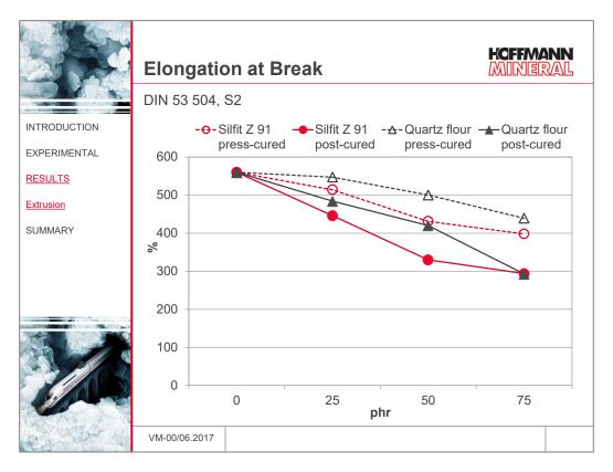
The post-cure gives rise to a decline of the elongation at break of the filler loaded compounds by 100 % (in absolute figures). With a loading of 25 resp. 75 phr, the difference between Silfit Z 91 and the quartz flour is not quite as pronounced as with 50 phr.
