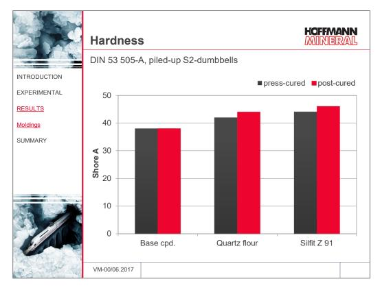
Both fillers, as expected, lead to a slight hardness increase of the base compound, while no significant difference can be detected between Silfit Z 91 and the quartz flour. With both fillers, post-curing further increases the hardness a little.
