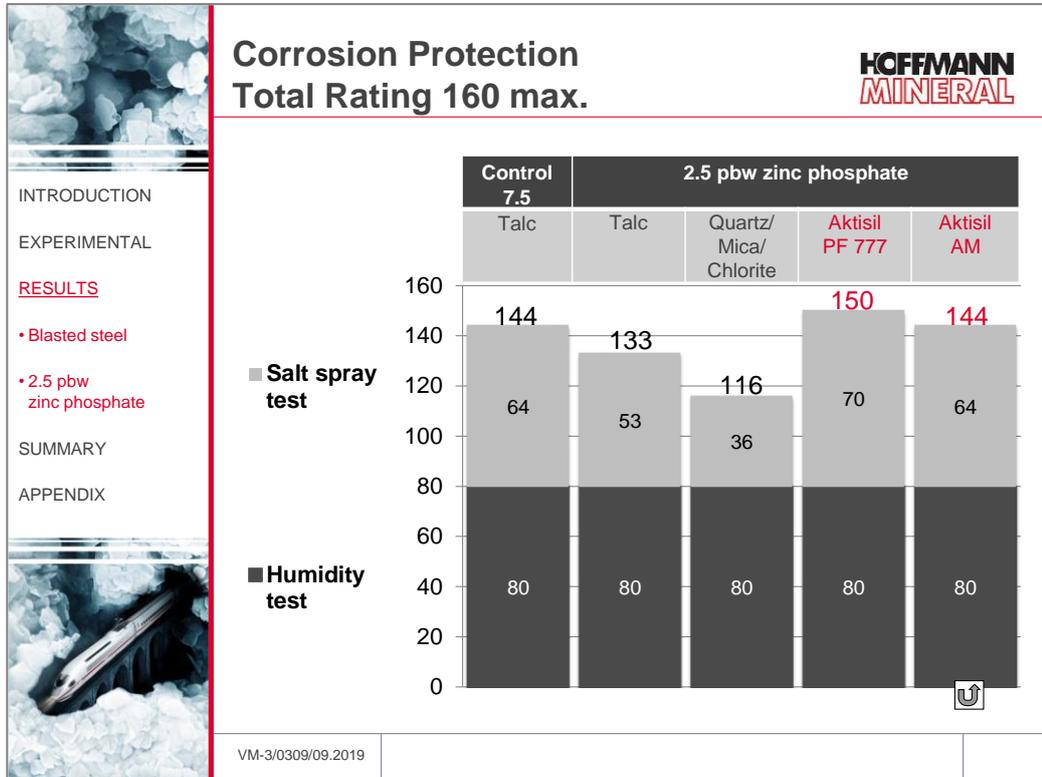
Fig. 27 blasted steel
