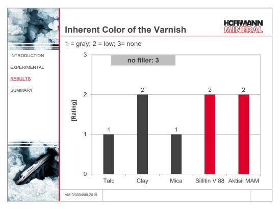
In the case of talc and mica, a distinct gray inherent color of the varnish occurred. With Neuburg Siliceous Earth and clay, the inherent color of the paint was significantly lower.
