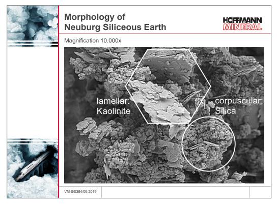
Aktisil products are made by modyfing the surface of Neuburg Siliceous Earth with chemical agents, mostly silanes. The by-products (for example alcohols) split off during the treatment reaction of the Aktisil grades are largely removed during the production process, which firmly attaches the silane to the filler surface. This helps minimize undesirable side effects, as they are potentially encountered with in-situ mixing (direct addition of silane to the compound).
