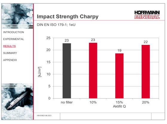
Despite the addition of Aktifit Q, impact strength remains approximately comparable to the unfilled control formulation without filler.
