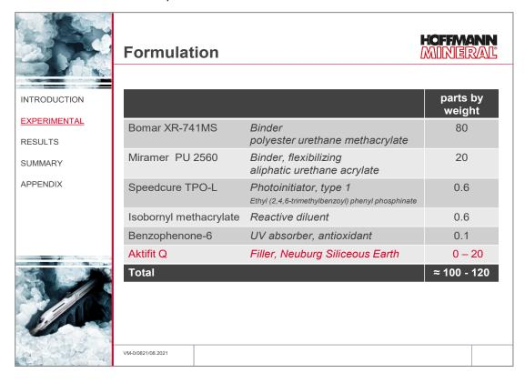
The main binder was Bomar XR-741MS, a high-viscosity polyester urethane methacrylate from Dymax. It is recommended for good heat deflection temperature, good adhesion and high hardness, as well as its resistance to yellowing.
