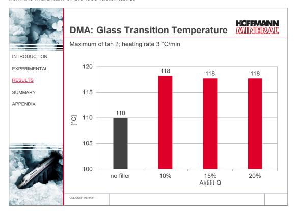
The addition of mineral filler leads to an increase of the glass transition temperature by approx. 8 °C (corresponds to approx. 7 %).
