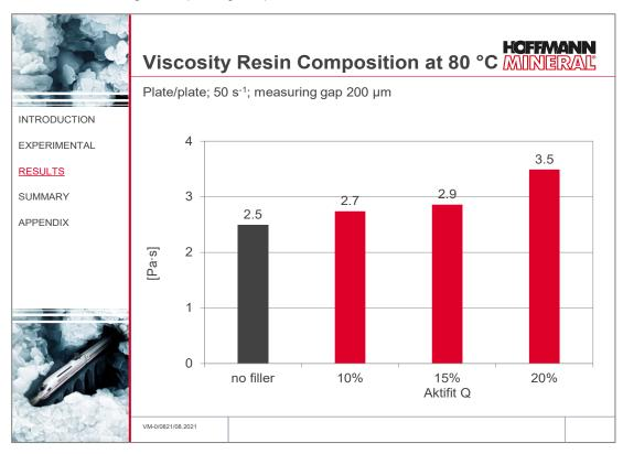
Depending on the filler dosage, a slight increase in viscosity of up to approx. 30% can be observed without negatively affecting the printing properties.
