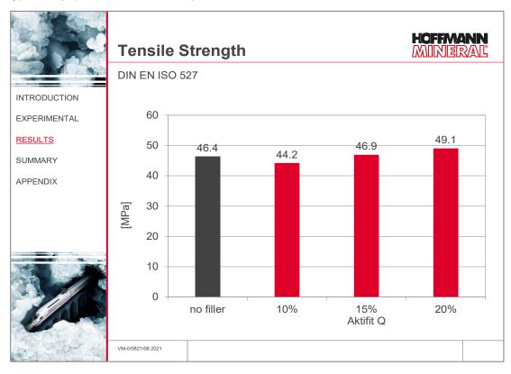
The tensile strength after the addition of Aktifit Q remains about on the level of the unfilled reference. At the highest dosage of 20 %, even a slight increase in strength can be observed.
