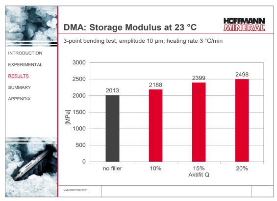
As expected, the stiffness of the specimens increases with increasing filler addition, up to  $25\,\%$  at  $20\,\%$  addition.
