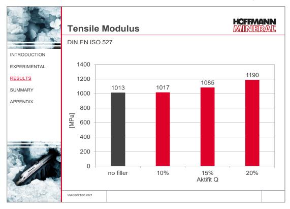
Analogously to the storage modulus, the increase in stiffness can be determined as a function of the filler addition, at 20 % filler addition approx. 17 %.
