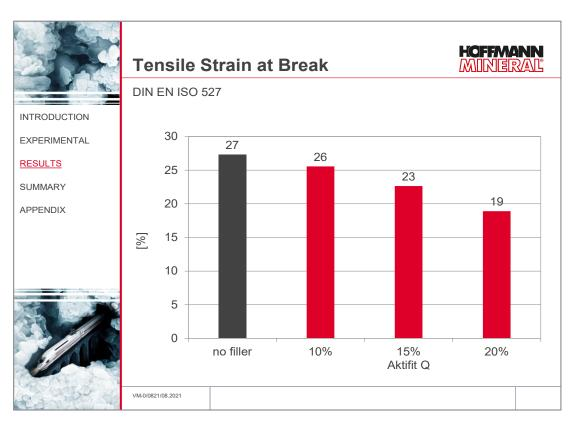
In contrast, the strain at break drops by up to 30 relative % depending on the filler loading, but remains at a good level of 19 % at the highest loading.
