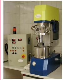
The compounds were prepared in a planetary mixer equipped with dissolver disc, kneading tool and scraper.
