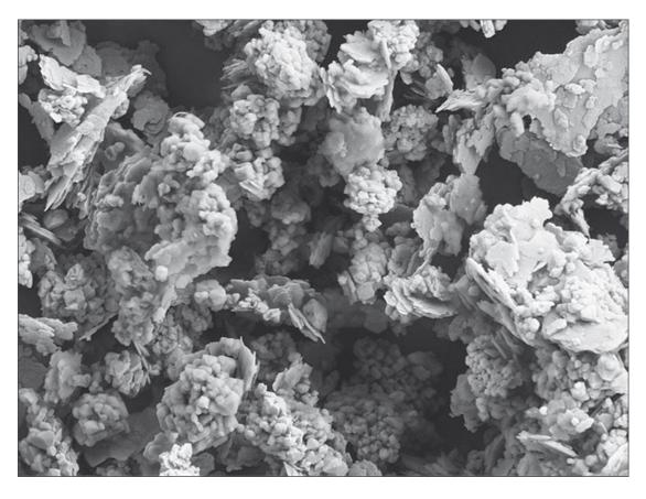
A natural combination of corpuscular Neuburg silica and lamellar kaolinite: a loose mixture impossible to separate by physical methods. The silica portion exhibits a round grain shape and consists of aggregated primary particles of about 200 nm diameter.
