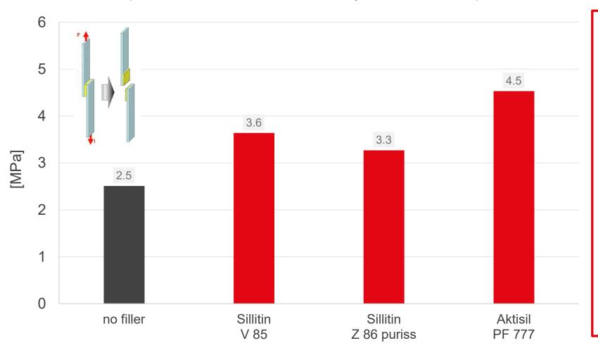
Neuburg Siliceous Earth results in a noticeable increased lap shear strength.
