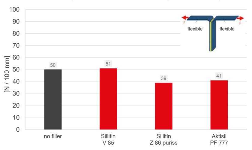
The peel resistance with Neuburg Siliceous Earth is approximately at the level of the unfilled formulation.
