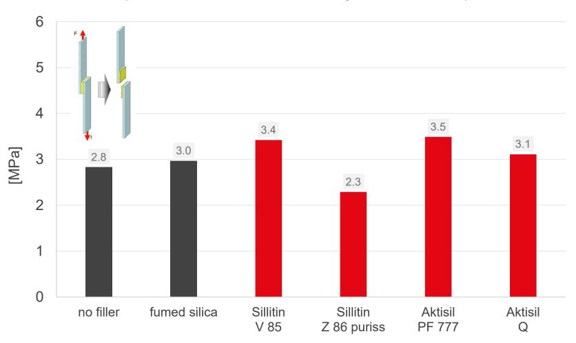
Neuburg Siliceous Earth results in a similar to slightly increased lap shear strength compared to the unfilled formulation or the competitor silica.
