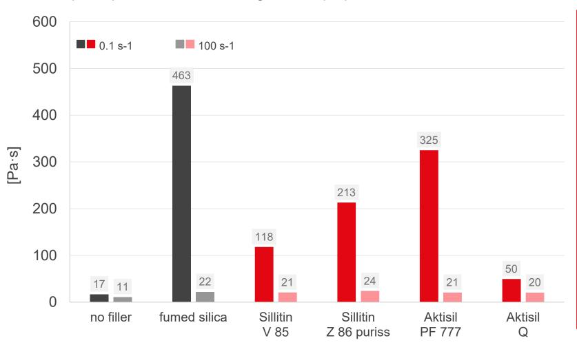
The addition of the filler increases the viscosity noticeably, especially in the low shear range.
