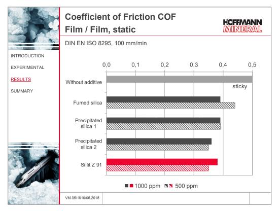
It proved practically impossible to determine the coefficient of friction film to film of the samples without mineral additive. The film sections tended too strongly to stick to each other (blocking). The addition of a mineral additive gives rise to a marked decrease of the COF film to film, but a dependence of the concentration could not be established. Silfit Z 91 at least comes out at the same level as the substantially more costly silicas.
