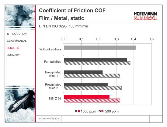
The addition of a mineral additive in the case of Silfit Z 91 and the two precipitated silicas leads to a concentration dependent, but marked reduction of the coefficient of friction between film and metal. Silfit Z 91 comes up with similar sliding properties as the precipitated silicas.
