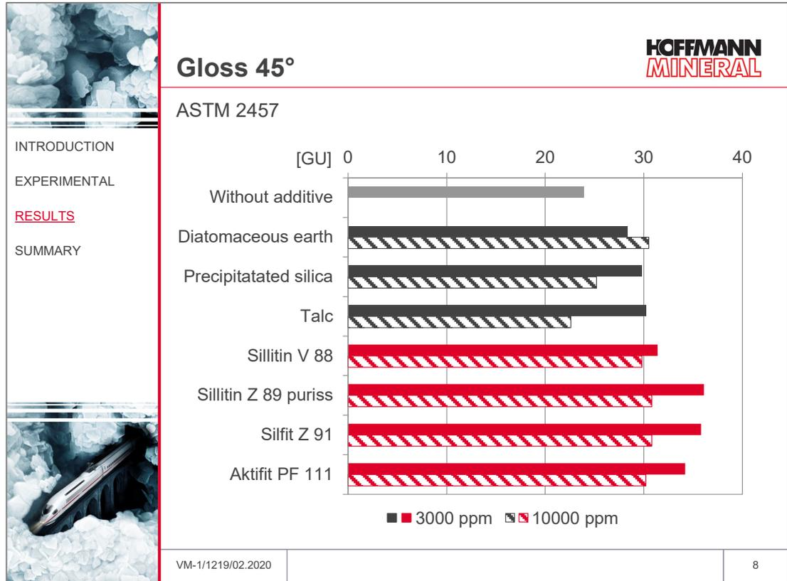
The use of 3000 ppm mineral additive noticeably increases the gloss of the film, with the fine grades of Neuburg Siliceous Earth achieving the highest values. Increasing the dosage to 10000 ppm reduces the gloss of talc and precipitated silica back to the level of the unfilled film. Diatomaceous earth and especially Neuburg Siliceous Earth in the higher dosage give films with higher gloss.
