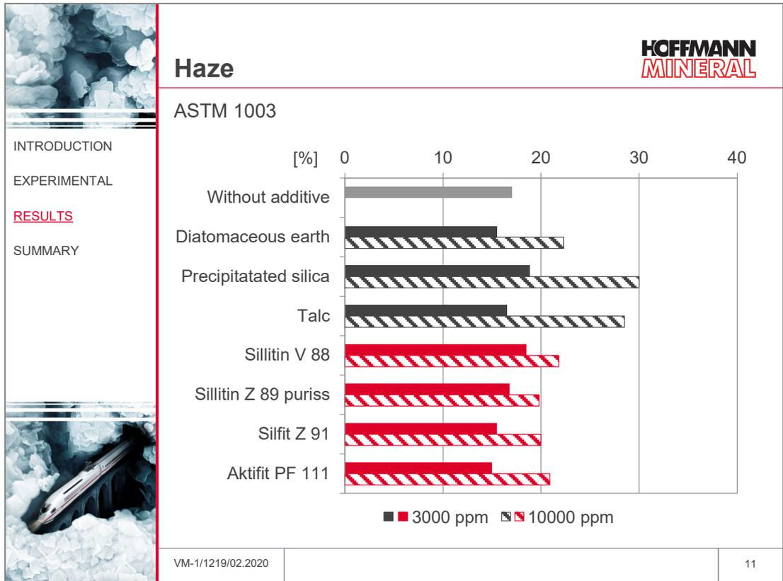
Analogous to the reduced image sharpness, the cloudiness caused by mineral additives increases accordingly in the higher dosage.
