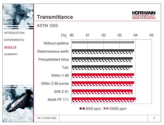
In the case of transmittance, there is a trend towards slightly lower values. In higher dosage, talcum reduces light transmission most significantly. Neuburg Siliceous Earth grades reach the highest values.
