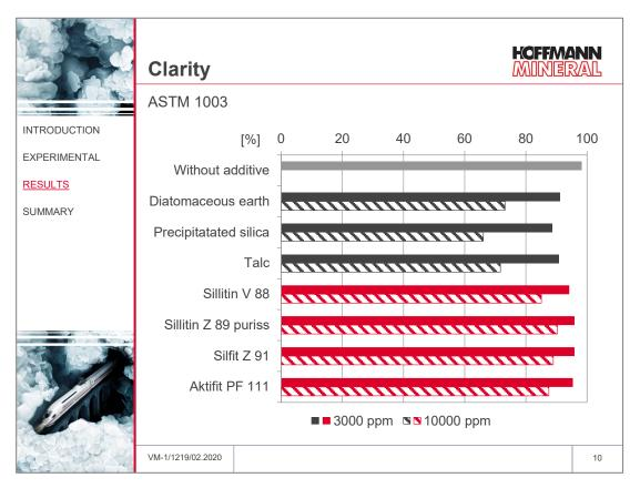
The addition of mineral additive results in a reduction of image sharpness for all materials, clearly visible in the higher dosage of 10000 ppm. With Neuburg Siliceous Earth, the image sharpness is significantly less affected than with the competing minerals, and in the low concentration the result of the film without additive is approached.
