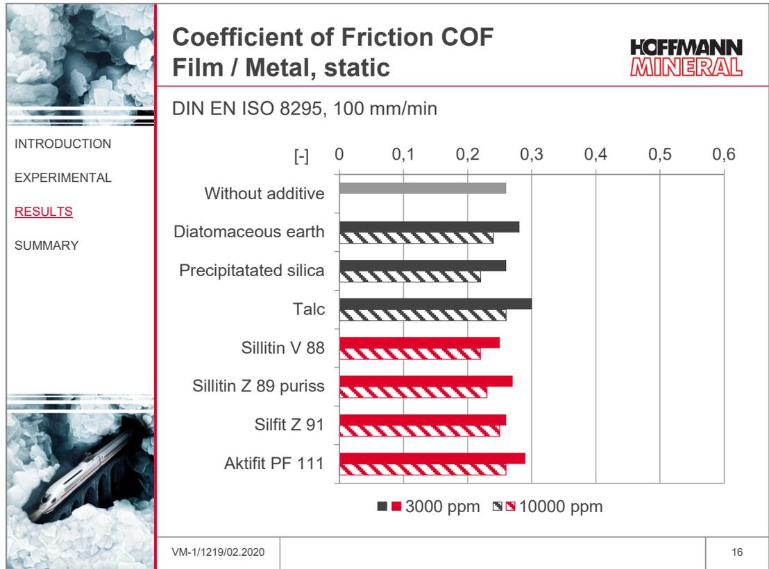
In the low dosage of 3000 ppm, the sliding properties film/metal are hardly influenced by the addition of the mineral additive and remain at the level of the unfilled film.
