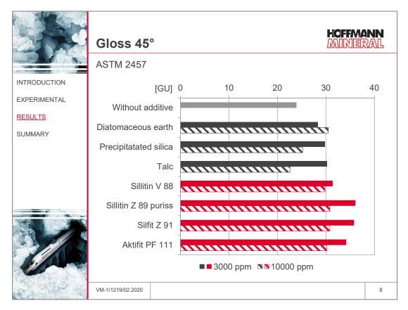
The use of 3000 ppm mineral additive noticeably increases the gloss of the film, with the fine grades of Neuburg Siliceous Earth achieving the highest values. Increasing the dosage to 10000 ppm reduces the gloss of talc and precipitated silica back to the level of the unfilled film. Diatomaceous earth and especially Neuburg Siliceous Earth in the higher dosage give films with higher gloss.
