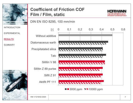
With regard to the coefficient of friction film/film, improved sliding properties can already be observed with the lower dosage of the mineral additive compared to the unfilled film. By increasing the dosage, this effect is even slightly enhanced. The finer grades of Neuburg Siliceous Earth, Sillitin Z 89 puriss, Silfit Z 91 and Aktifit PF 111, show the best results here. The coarser Sillitin V 88 is better suited for thicker films.
