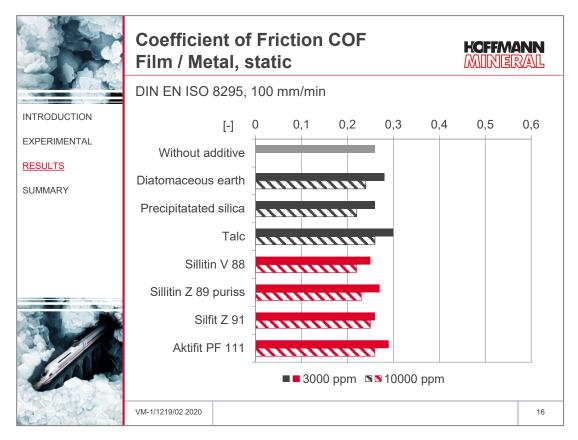
In the low dosage of 3000 ppm, the sliding properties film/metal are hardly influenced by the addition of the mineral additive and remain at the level of the unfilled film.
