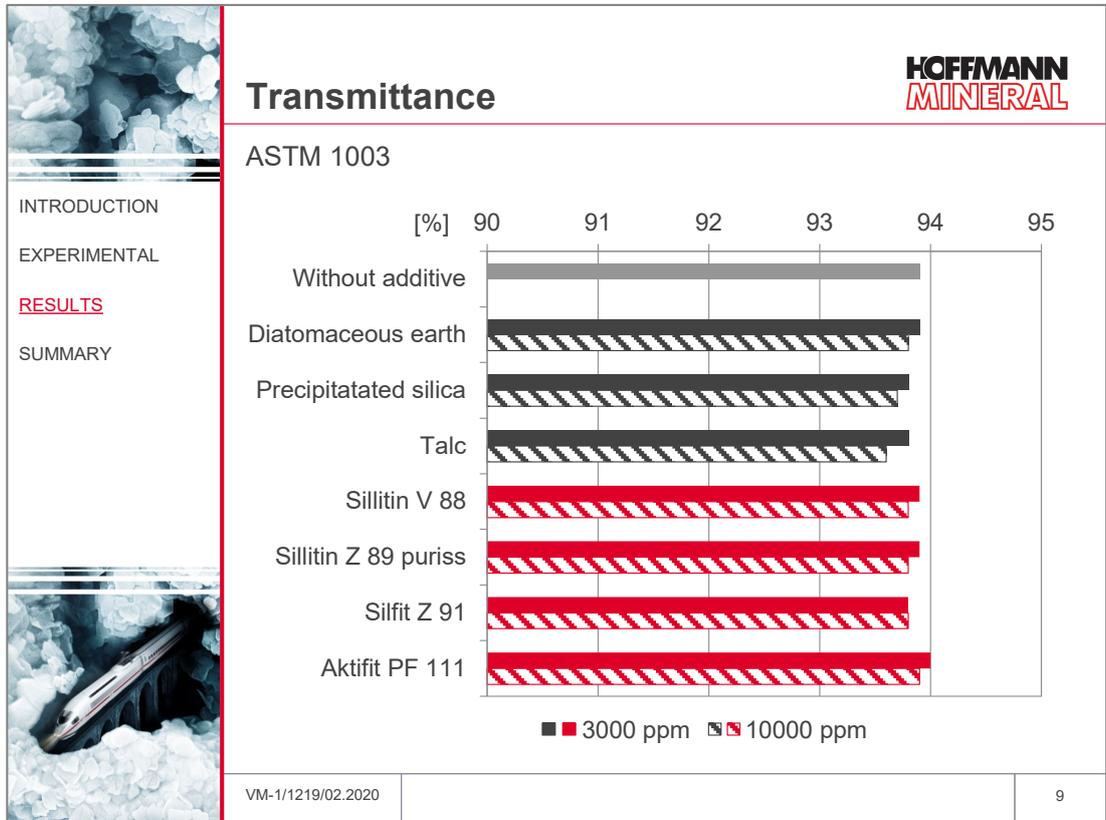
In the case of transmittance, there is a trend towards slightly lower values. In higher dosage, talcum reduces light transmission most significantly. Neuburg Siliceous Earth grades reach the highest values.
