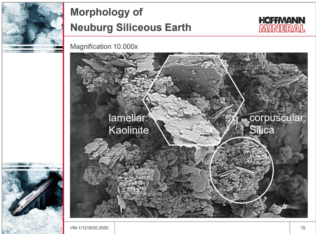
The basis for the calcined Neuburg Siliceous Earth is the standard product Sillitin Z 86. In a thermal process, the water of crystallization in the kaolinite portion is removed and new, largely amorphous mineral phases are formed.
