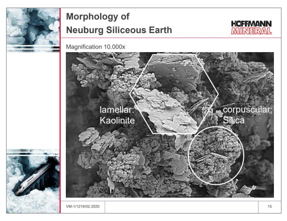
The basis for the calcined Neuburg Siliceous Earth is the standard product Sillitin Z 86. In a thermal process, the water of crystallization in the kaolinite portion is removed and new, largely amorphous mineral phases are formed.
