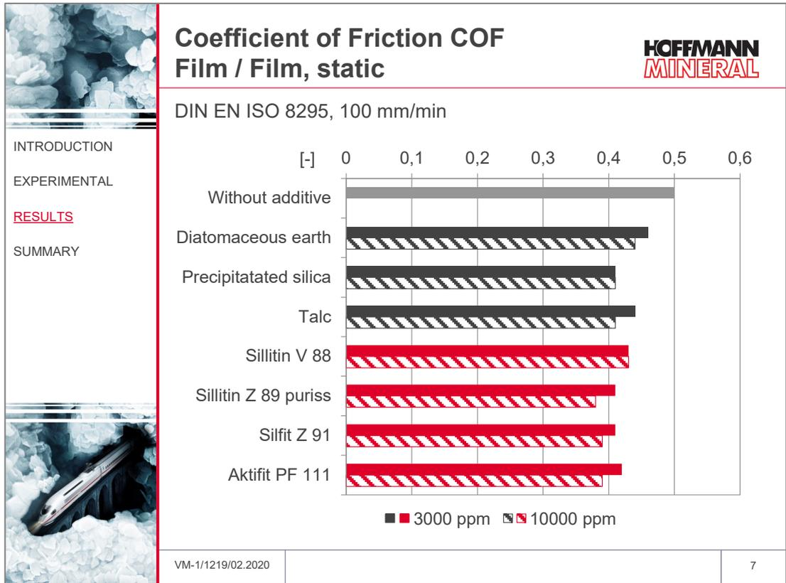
With regard to the coefficient of friction film/film, improved sliding properties can already be observed with the lower dosage of the mineral additive compared to the unfilled film. By increasing the dosage, this effect is even slightly enhanced. The finer grades of Neuburg Siliceous Earth, Sillitin Z 89 puriss, Silfit Z 91 and Aktifit PF 111, show the best results here. The coarser Sillitin V 88 is better suited for thicker films.
