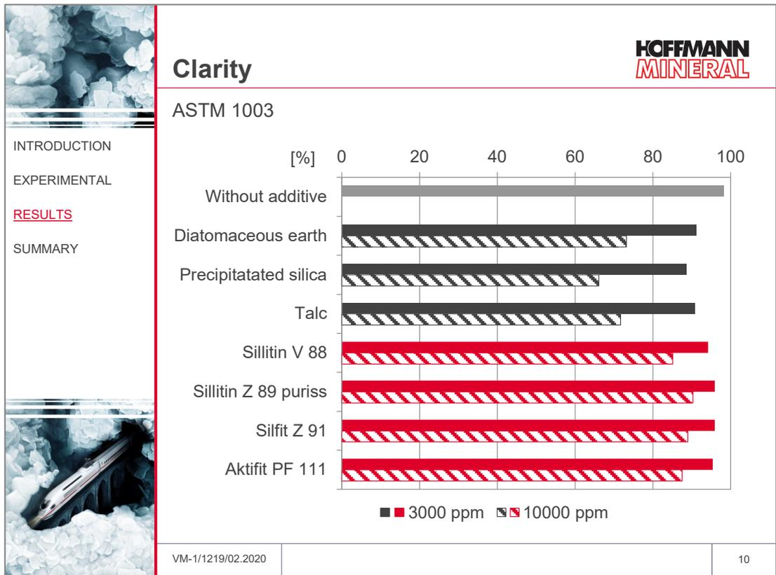
The addition of mineral additive results in a reduction of image sharpness for all materials, clearly visible in the higher dosage of 10000 ppm. With Neuburg Siliceous Earth, the image sharpness is significantly less affected than with the competing minerals, and in the low concentration the result of the film without additive is approached.
