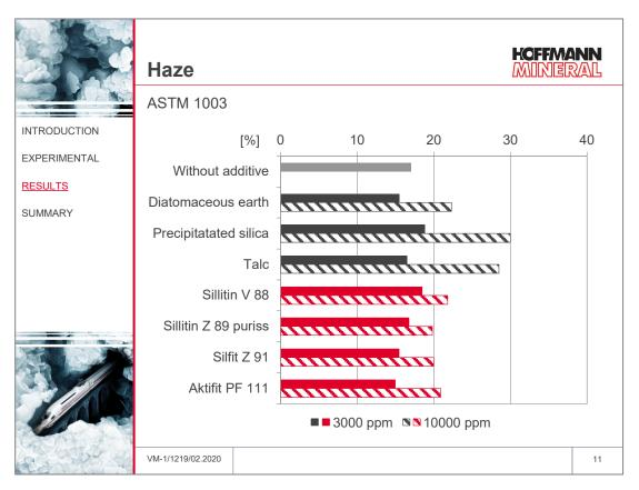
Analogous to the reduced image sharpness, the cloudiness caused by mineral additives increases accordingly in the higher dosage.
