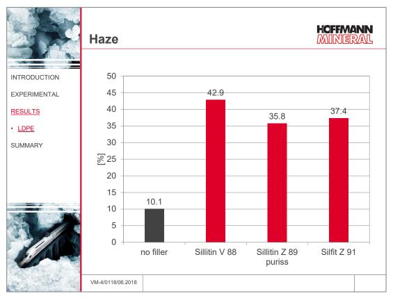
Film haze proved to be similar to the diffuse transmission proportion. The film without filler was relatively clear, as expected, with 10 % haze, whereas the haze increased strongly with the addition of fillers. However, the finer filler particles in Sillitin Z 89 puriss and Silfit Z 91 caused less haze than the coarser particles in Sillitin V 88.
