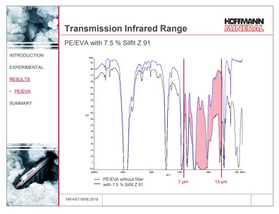
Adding filler significantly improves the barrier performance of the film. As was also the case with the LDPE film, Sillitin Z 89 puriss with its fine particles reduced transmission more strongly in the range of less than 9  $\mu$ m compared to the coarser Sillitin V 88, while calcined Silfit Z 91 tended to reduce transmission more strongly in the 11-12  $\mu$ m range.
