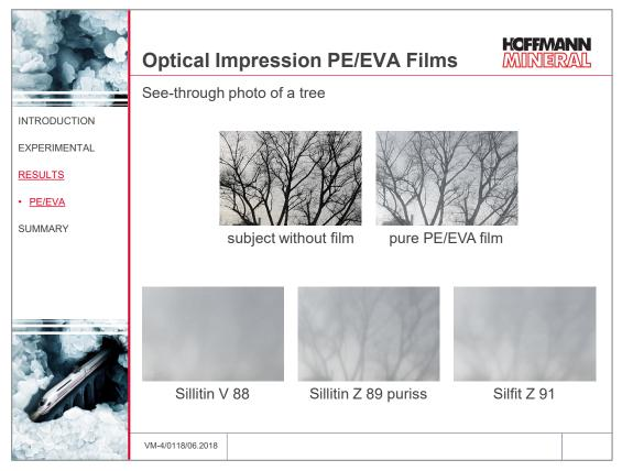
The optical impression of the PE/EVA films is more or less as expected, based on the measured haze properties. Of the films with filler, the film with Sillitin Z 89 puriss again shows the clearest and the film with Sillitin V 88 the milkiest picture.
