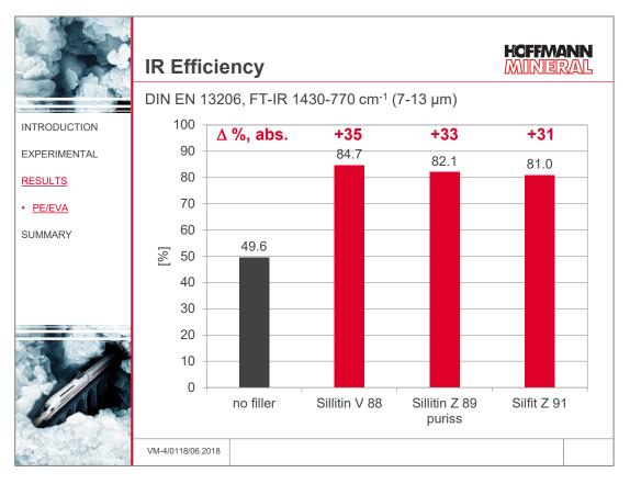
The efficiency of pure PE/EVA film is already approx. 50 %. By adding filler, this performance can be enhanced by further 30-35 % to approx. 80-85 %.
