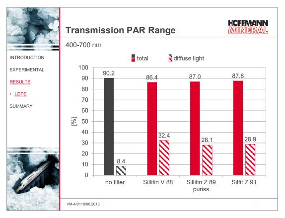
As expected, the film without filler demonstrated the highest total transmission. The addition of filler only reduces transmission marginally – the loss when using the finer fillers Sillitin Z 89 puriss and Silfit Z 91 is slightly less than that caused by the coarser Sillitin V 88.
