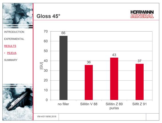
Gloss measured at an incident angle of 45° dropped as a result of adding the filler by approx. 20-30 units – the films with filler are more mat than the film without.
