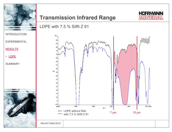
The barrier performance of Silfit Z 91 is also good, and stronger in the 11-12  $\mu$ m range than Sillitin Z 89 puriss with virtually the same fine particle size. Thermal post-treatment is probably the explanation for this difference.
