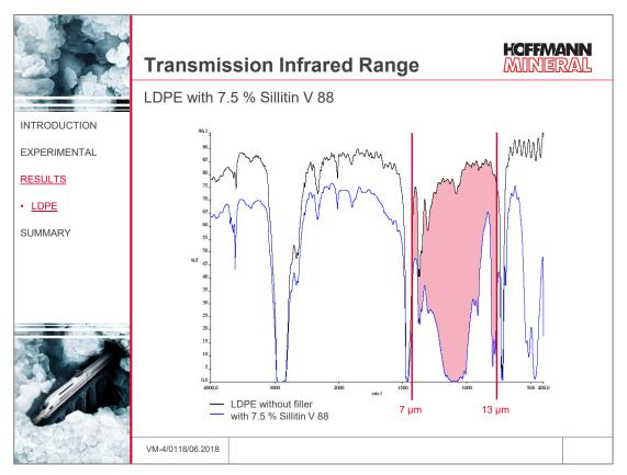
Compared to the unfilled film, Sillitin V 88 significantly reduces transmission in the near- and mid-infrared range.
