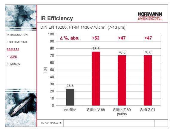
Unlike the pure PE film with its efficiency of just 24 %, the barrier performance of the mineral filler is 70-75 %. As such, the films with filler have substantially better thermal retention capability.
