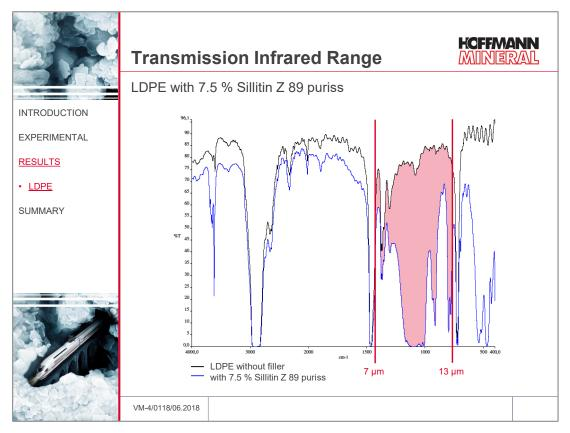
A clear IR radiation barrier effect is also discernible with Sillitin Z 89 puriss. Compared to Sillitin V 88, however, Sillitin Z 89 puriss raises the barrier effect in the shorter wave range < 9  $\mu$ m, which can be explained by the finer particle size.
