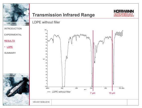
The IR radiation barrier effect demonstrated by the LDPE film without filler was low in the relevant wavelength range.
