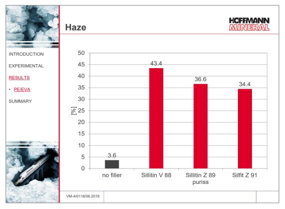
The haze of the film without filler was only approx. 4 %, as expected. Haze increases strongly with the addition of the fillers, whereby it is again the finer filler particle size of Sillitin Z 89 puriss and Silfit Z 91 that produces less haze than the coarser particles in Sillitin V 88.
