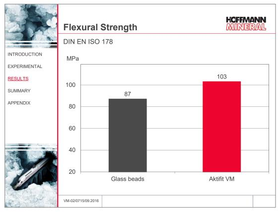
The flexural strength with Aktifit VM is higher by 18 % compared with the glass beads; which is in agreement with the results for the tensile strength.
