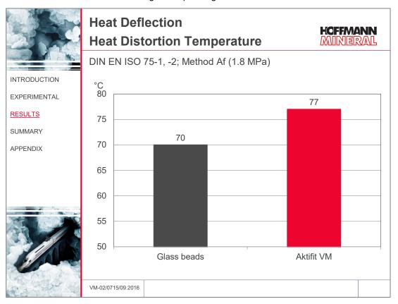
With Aktifit VM the HDT is somewhat higher than with the glass beads, and consequently the compound offers a slightly improved dimensional stability at higher temperature.
