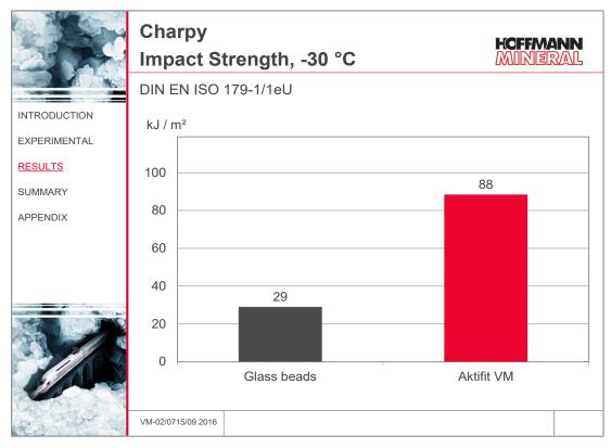
The same situation is true at low temperature (-30  $^{\circ}$ C): the compound with Aktifit VM shows an impact strength several times higher.
