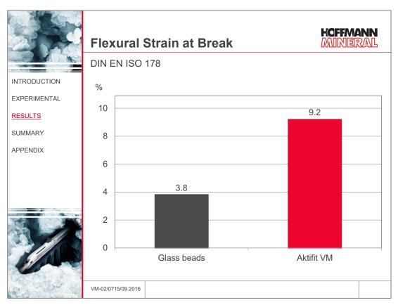
Also in the bending tests the samples with Aktifit VM break at about twice the elongation compared with the glass beads.
