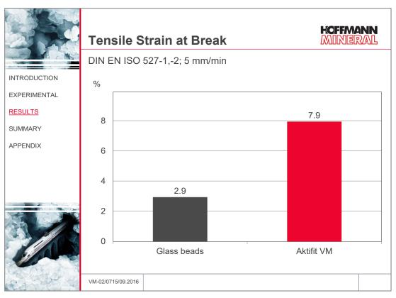
In comparison with the competitive filler, the samples filled with Aktifit VM only break at about the double strain. This effect is welcome for applications where building parts when mounted have to resist to certain deformations, as for example snap hook joints.
