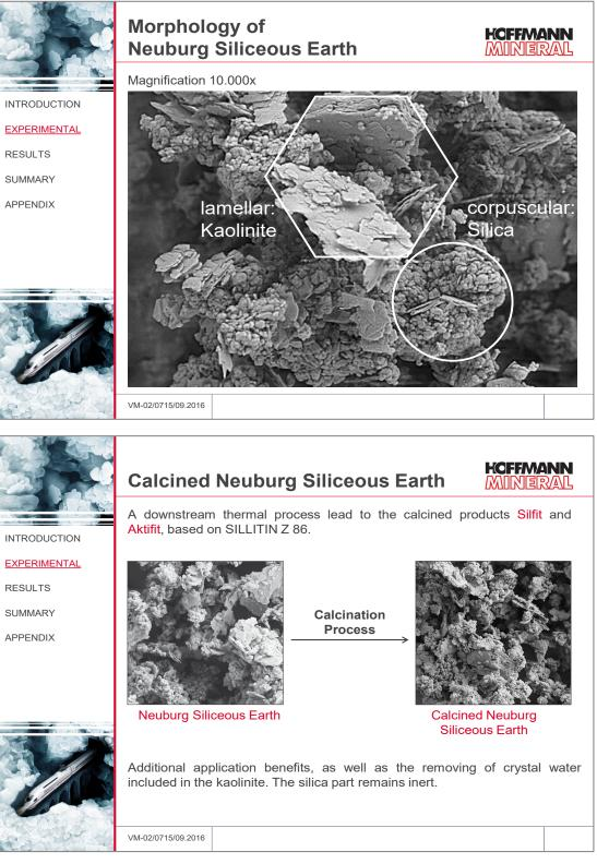
During calcination, Neuburg Siliceous Earth is subjected to a heat treatment. The components and the thermal process lead to a product that offers special performance benefits as a functional filler.
