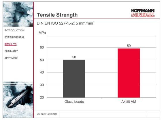
The tensile strength obtained with Aktifit VM is approximately 18 % higher than with the glass beads.
