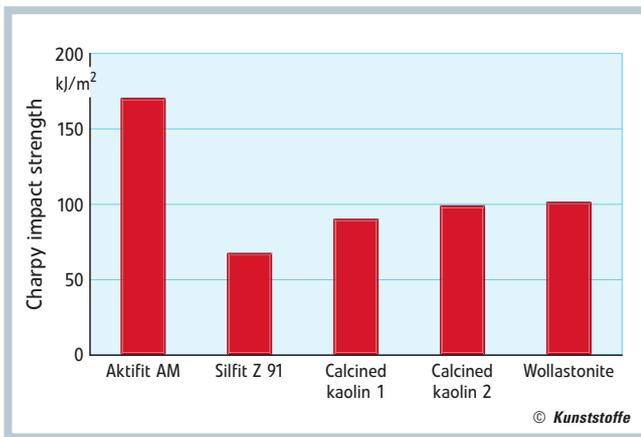
**Fig. 5.** In the test for Charpy impact strength with the 15 J pendulum, too, the polyamide compound containing Aktifit AM, showed an impact strength significantly above that of the competitor fillers
