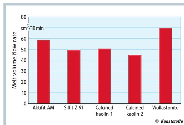
**Fig. 1.** The melt flow of polyamide compound containing Aktifit AM did not quite reach the level of the compound filled with wollastonite, but was significantly above the values of the tested compounds with kaolin
