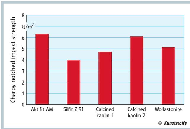
**Fig. 3.** The value for the Charpy notch impact strength of polyamide compounds with Aktifit AM slightly exceeds the value for kaolin 2 compounds, but significantly surpasses that of kaolin 1 and wollastonite compounds
