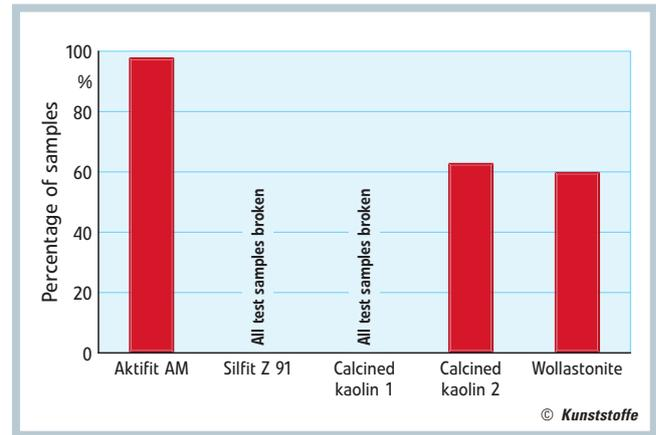
**Fig. 4.** The percentage of unbroken samples for Charpy impact strength with a 4 J pendulum containing Aktifit AM, resulted in almost 100 %, thus significantly outperforming the competitor materials
