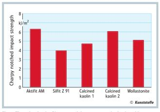
Fig. 3. The value for the Charpy notch impact strength of polyamide compounds with Aktifit AM slightly exceeds the value for kaolin 2 compounds, but significantly surpasses that of kaolin 1 and wollastonite compounds
