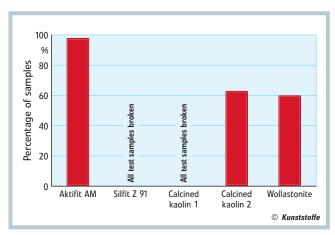
Fig. 4. The percentage of unbroken samples for Charpy impact strength with a 4 J pendulum containing Aktifit AM, resulted in almost 100 %, thus significantly outperforming the competitor materials
