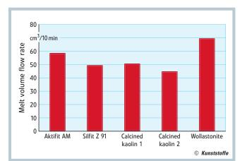
Fig. 1. The melt flow of polyamide compound containing Aktifit AM did not quite reach the level of the compound filled with wollastonite, but was significantly above the values of the tested compounds with kaolin
