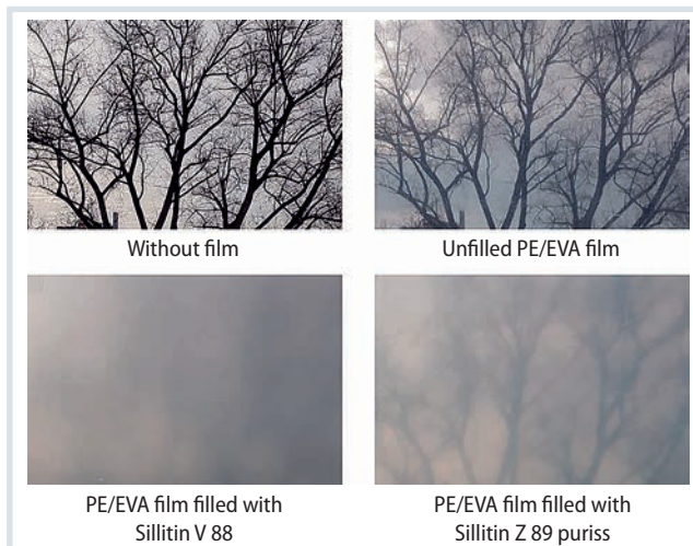
Fig. 5. The fillers also confer a milkier appearance on PE/EVA film. In these cases, too, the appearance and haze depends on the size of the filler particles.
