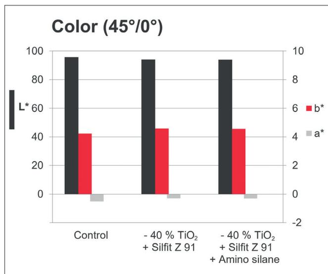
Figure 1. Colour ratio after partial TiO<sub>2</sub> replacement at a wet film thickness (WFT) of 600µm
