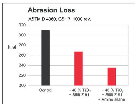
Figure 3. Abrasion resistance after partial TiO<sub>2</sub> replacement with Silfit Z 91 pure and Silfit Z 91 + amino silane
