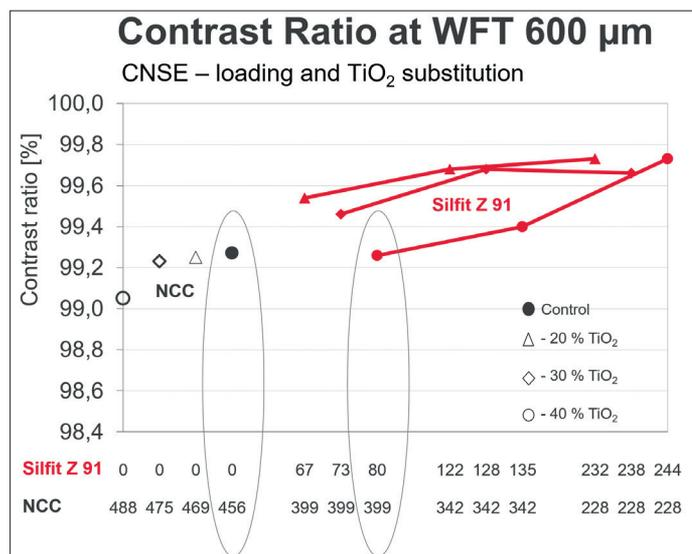
Figure 2. Contrast ratio after partial TiO<sub>2</sub> replacement at a WFT of 600µm
