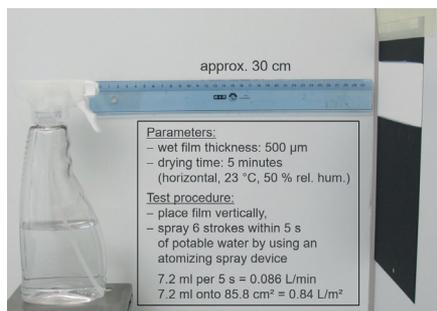
Figure 4. Testing set-up for the early rain resistance measurement
