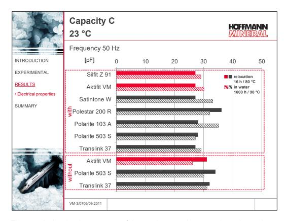
The capacity is related to geometry of the specimens and must not be understood as a material constant. Since the dielectric constant  $\epsilon_R$  is a factor for the calculation of the capacity and the specimen dimensions were widely constant, these two electrotechnical parameters correlate well with each other.
