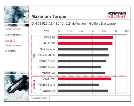
The calcined Neuburg Siliceous Earth grades attain higher Vulcameter torque maxima compared to the other fillers tested.
