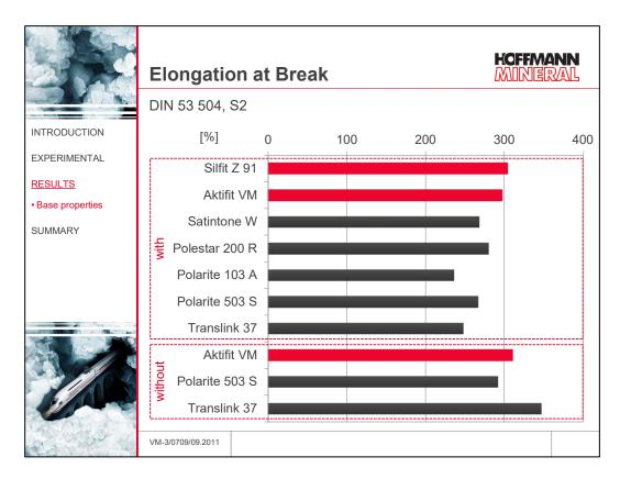
The elongation at break levels obtained with calcined Neuburg Siliceous Earth are somewhat higher than those realized especially with the surface treated calcined clays. Without the in situ added vinyl silane, the results move closer to each other.
