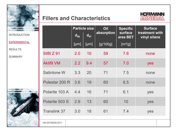
Silfit Z 91 and Aktifit VM were evaluated in comparison with surface treated and untreated calcined clays.
