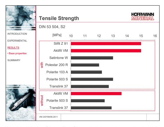
The calcined Neuburg Siliceous Earth fillers attain higher tensile strength levels with but also without in situ added vinyl silane. As evident from the graph, already the untreated Silfit Z 91 gives a higher tensile strength than all other competitive fillers tested. The same is true for Aktifit VM.
