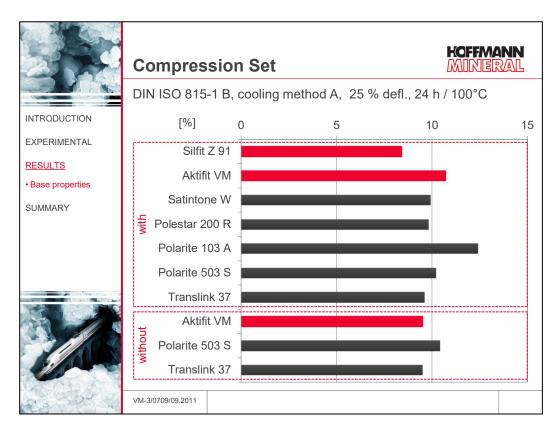
The compression set does not represent an immediate characteristic of cable insulation compounds but it gives indications about the capacity for elastic recovery after deformation. The selection of fillers shows no remarkable effect on the compression set. With all fillers tested very similar results are obtained.
