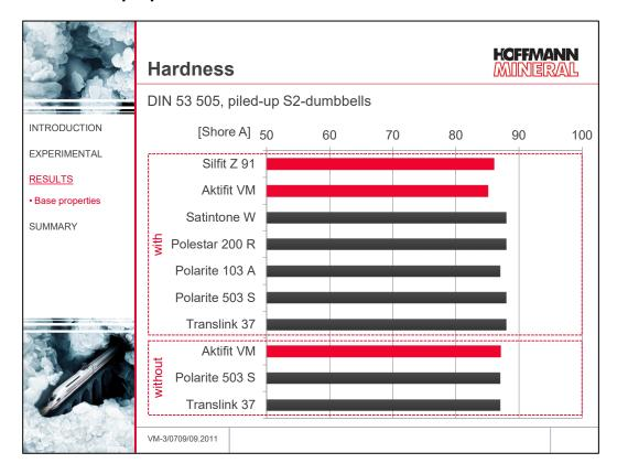
Hardness was determined on three piled-up S2 dubbell specimens. No significant hardness differences are seen between the individual filler. Even taking out the in situ added vinyl silane does not affect the results.
