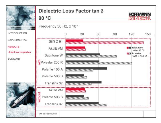
As the usual service temperature of medium and high voltage cables is around 90  $^{\circ}$ C, the dielectric loss factor was also determined on samples at 90  $^{\circ}$ C. The industry standard of the dielectric loss factor is about 30 x 10<sup>-4</sup>.
