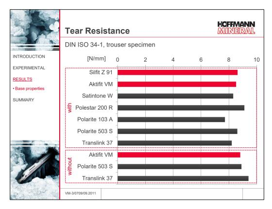
Likewise, for tear resistance no differences can be observed - neither between the individual fillers nor for the presence respectively absence of added vinyl silane.
