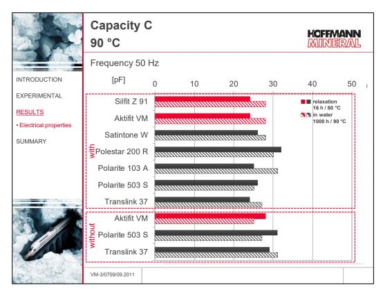
At a temperature of 90  $^{\circ}$ C - which is the usual service temperature - no marked differences can be found between the variations. Nevertheless it should be noticed here that the results for Silfit Z 91 and Aktifit VM are mostly at the lower end and thus better.
