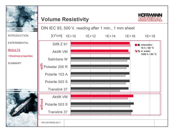
As the graph for the dry results (after relaxation) shows, the calcined Neuburg Siliceous Earth grades impart high volume resistivites which are on one level with the calcined clay as usually applied in this application.
