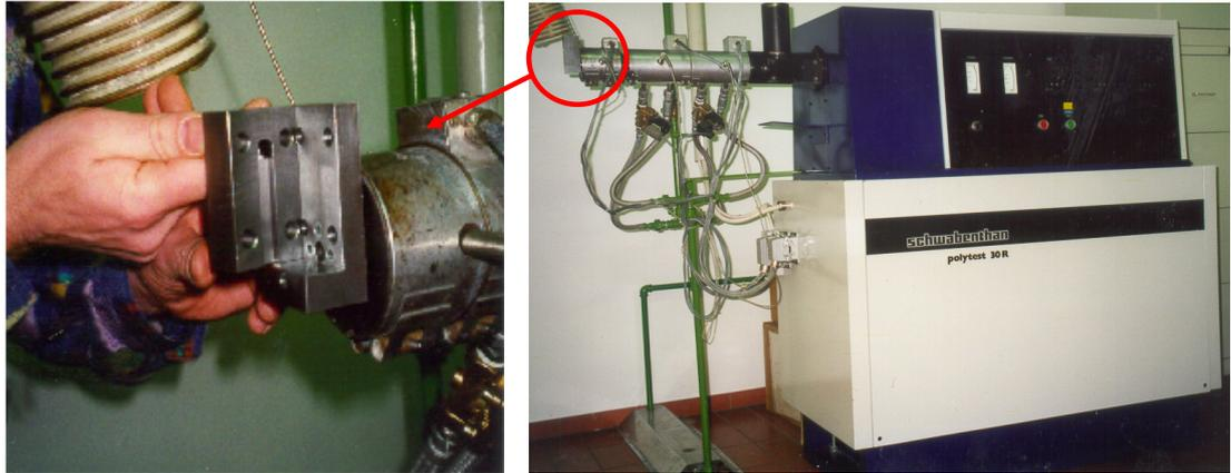
**Figure 1:** Special front-end test device and Schwabenthan extruder Polytest 30 R
