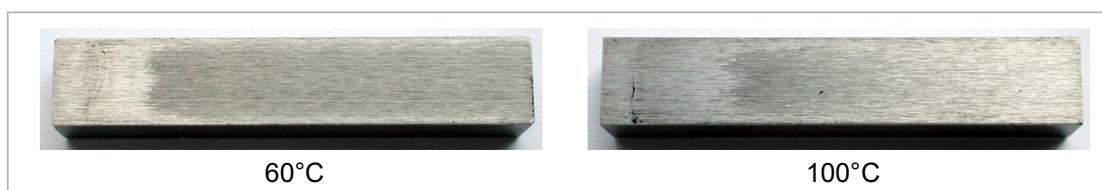
**Figure 6:** Effect of extruder head temperature on the die-plating effect
