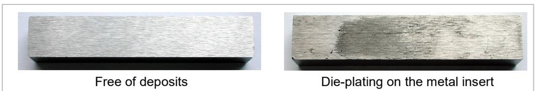
**Figure 3:** Examples for different die-plating tendency
