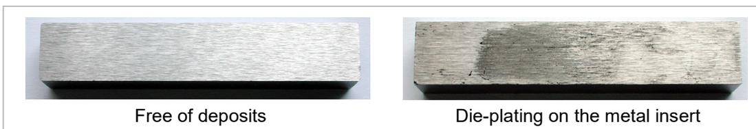
**Figure 3:** Examples for different die-plating tendency
