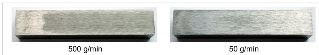
**Figure 5:** Effect of extrusion throughput on the die-plating effect
