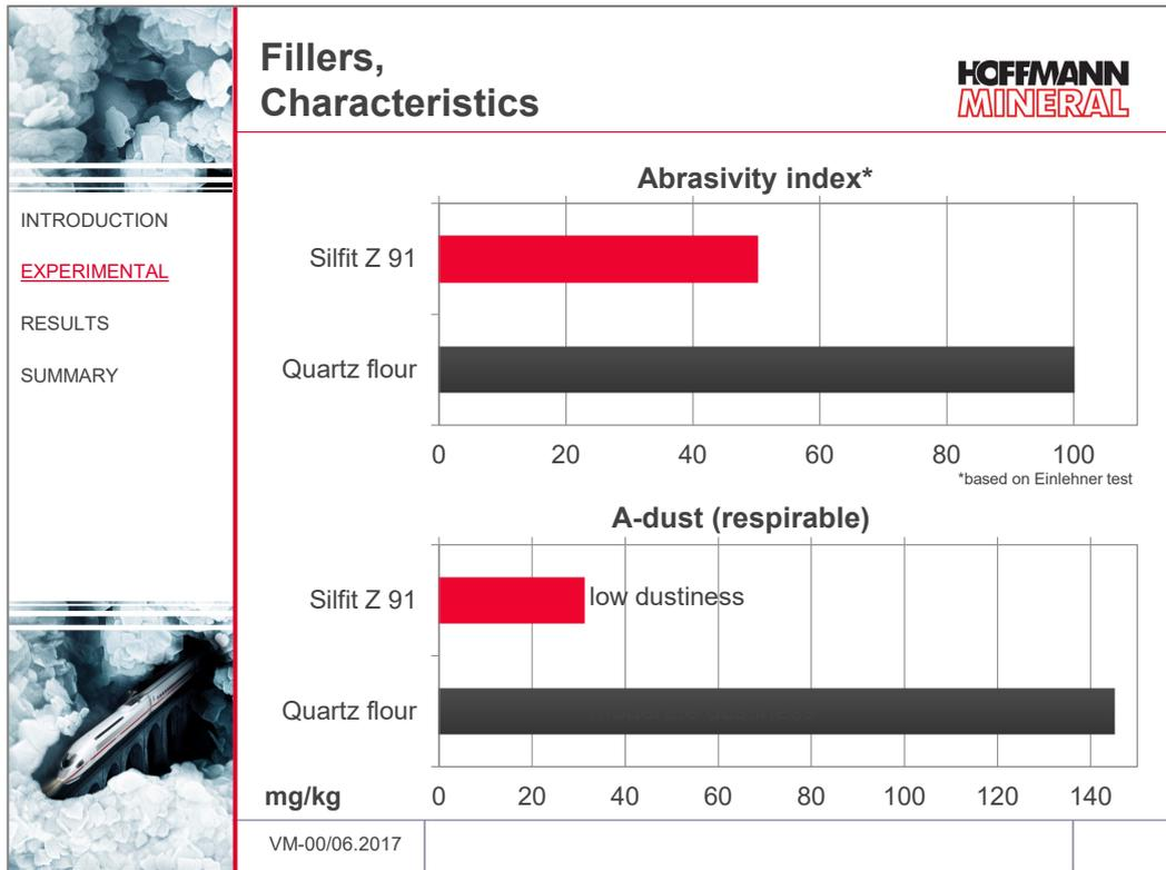
With the help of the Einlehner test which allows to assess the wear of processing machines etc., it can be confirmed that Silfit Z 91 offers a marked improvement over the quartz flour with respect to abrasivity.
