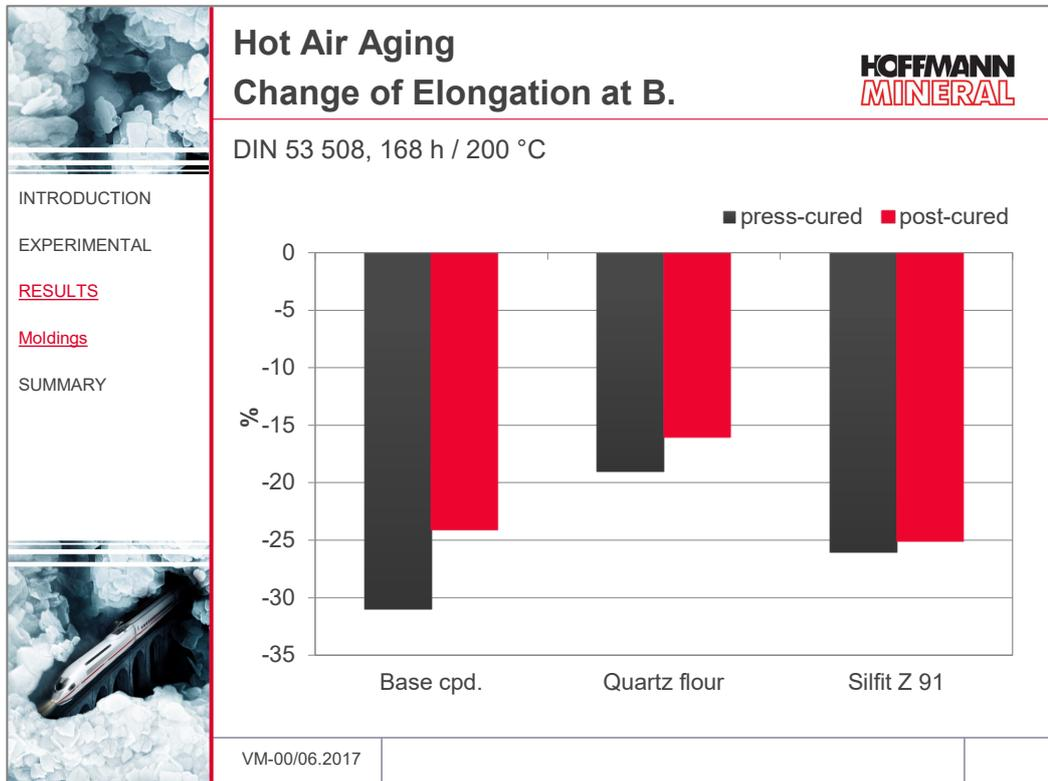
While the quartz flour addition results in a somewhat smaller change of the elongation at break during hot air aging, Silfit Z 91 remains practically on level with the base compound.
