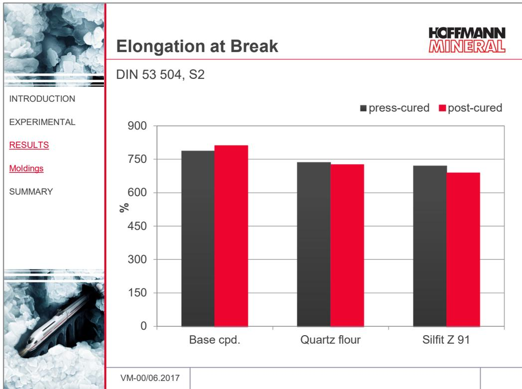
The elongation at break with 25 phr filler is only marginally lower compared with the base compound. The choice of the filler has no significant influence on the results, as little as the post-curing step.
