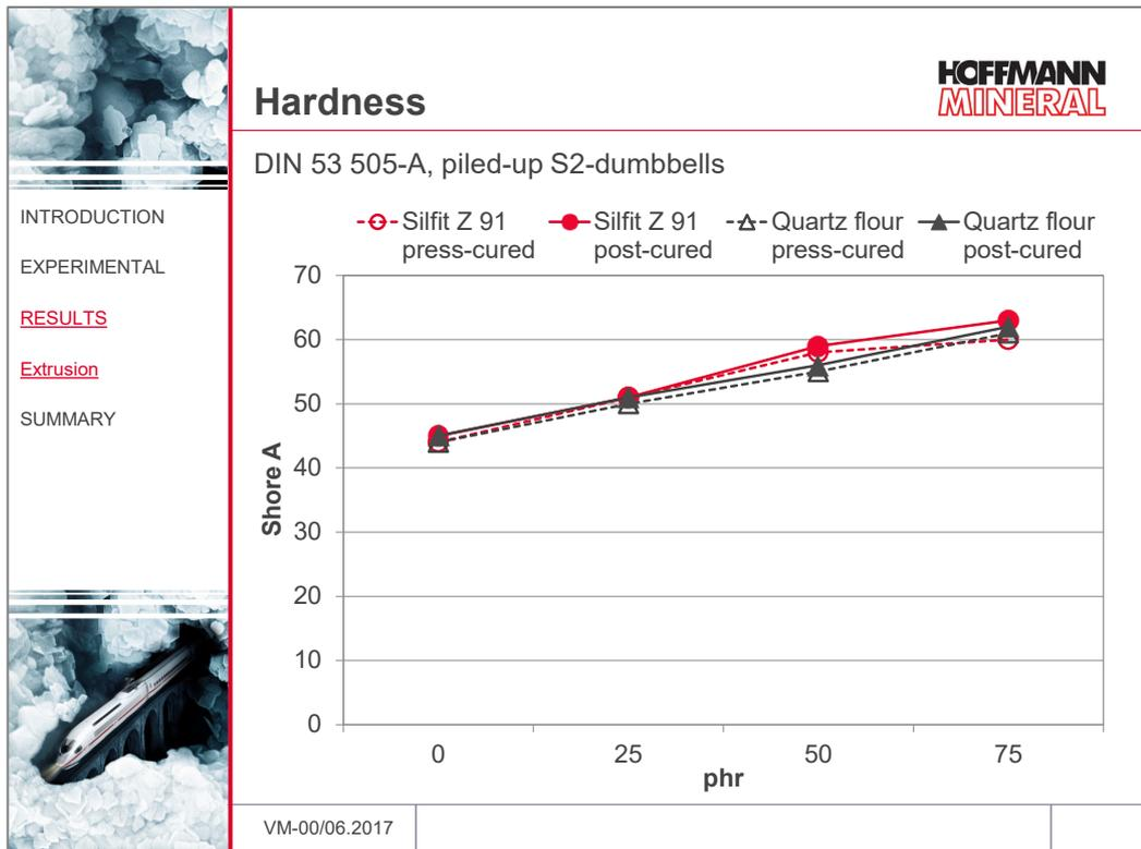
The stepwise increase of the filler loading for Silfit Z 91 and the quartz flour gives rise to comparable increases in hardness. A post-cure exerts no significant influence, neither with Silfit Z 91 nor with quartz flour.
