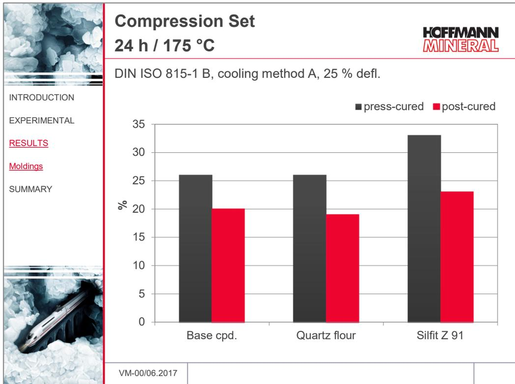
By post-curing, the compression set with Silfit Z 91 can be decreased in a way that the results arrive at a comparable level with the unfilled base compound or the quartz flour.
