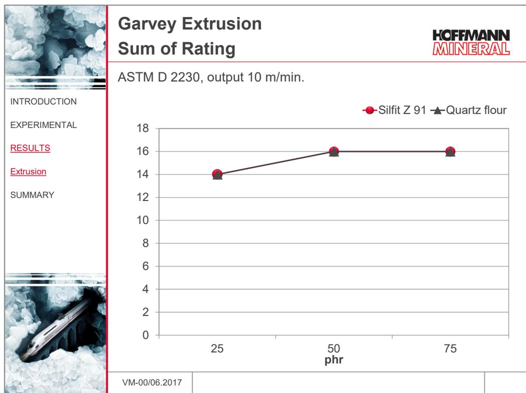
With a constant output rate of 10 m/min., no differences can be discovered between the extrudates filled with Silfit Z 91 resp. with the quartz flour.
