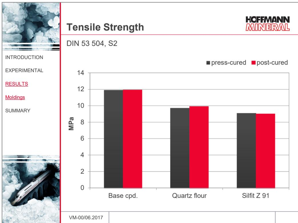
By adding the fillers, the tensile strength of the base compound is somewhat reduced. The compounds filled with Silfit Z 91 give rise to only marginally lower levels than those with quartz flour. Post-curing here shows practically no effect.
