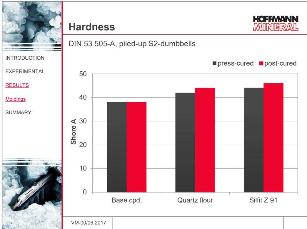
Both fillers, as expected, lead to a slight hardness increase of the base compound, while no significant difference can be detected between Silfit Z 91 and the quartz flour. With both fillers, post-curing further increases the hardness a little.
