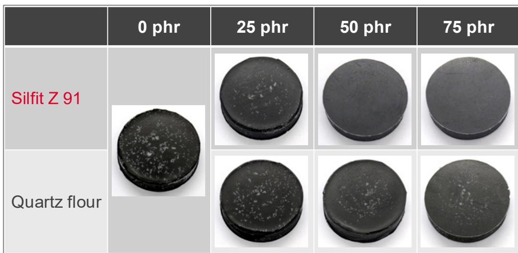
It becomes quickly clear that Silfit Z 91 at a loading level of 25 phr already gives rise to a marked reduction of the blooming. From 50 phr upwards, the blooming is completely eliminated.
