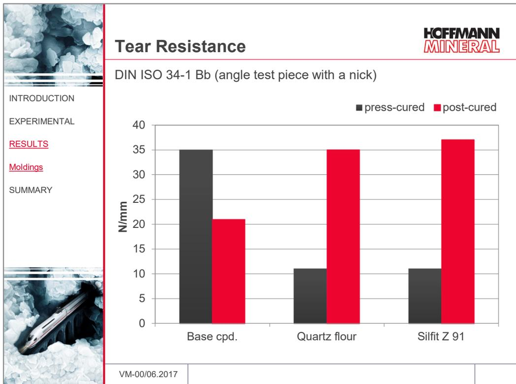
While the tear resistance of the base compound reacts negatively on the post-cure, the results of the compounds with Silfit Z 91 resp. quartz flour come out distinctly higher. A significant difference between the two fillers cannot be detected.
