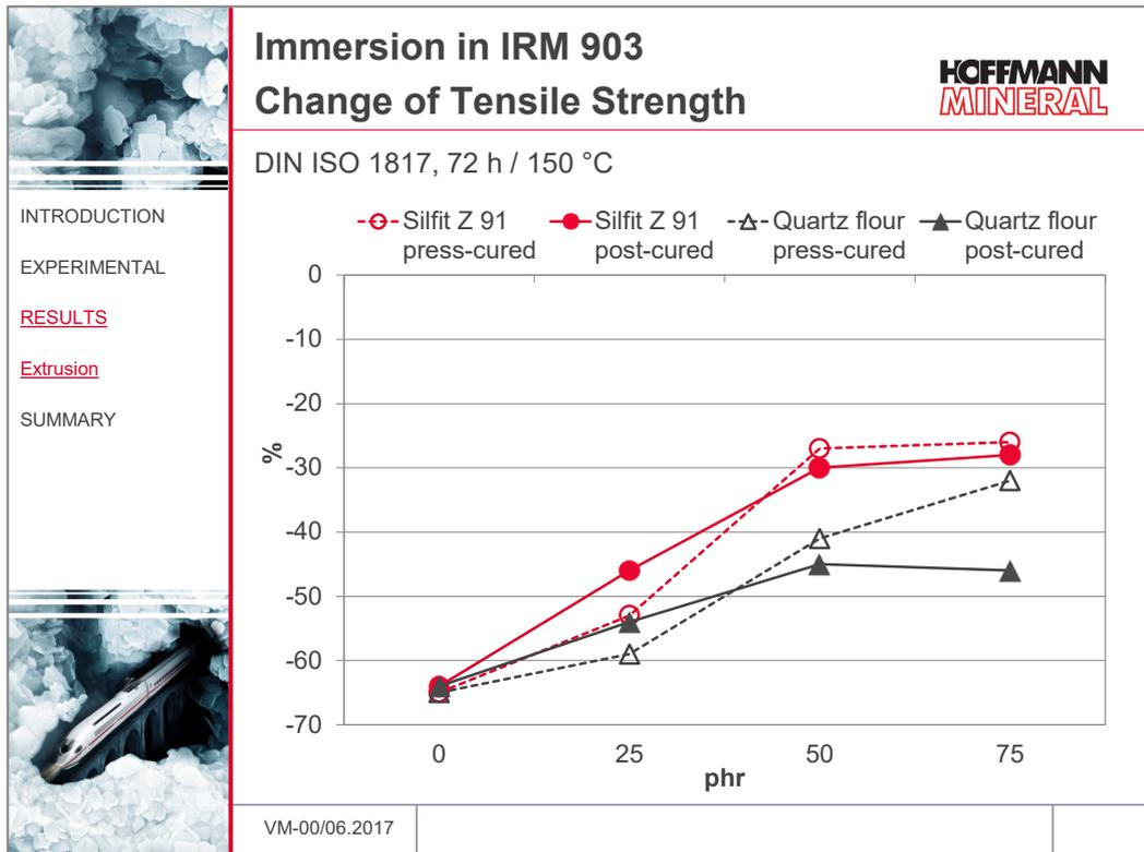
While the volume change upon immersion in reference oil IRM 903 of compounds loaded with Silfit Z 91 does not show any differences vs. those with quartz flour, with respect to changes in tensile strength they give proof of advantages. In fact, the tensile strength results of the press-cured as well as of the post-cured samples with Silfit Z 91 drop less than with quartz flour.
