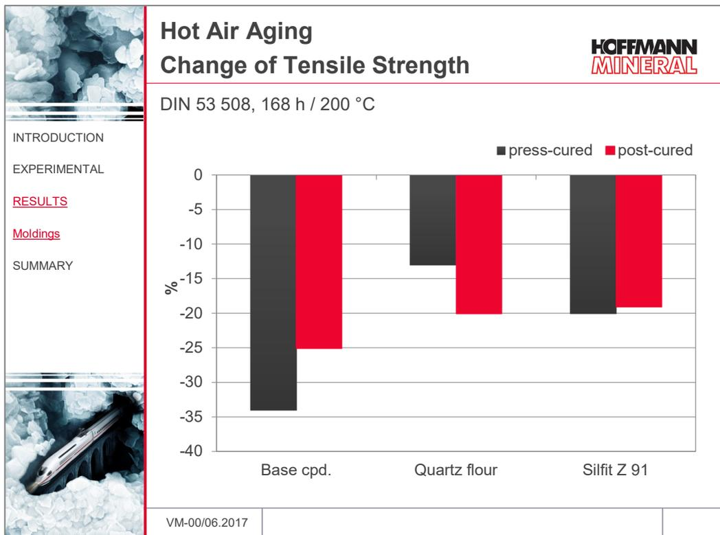
The changes of the tensile strength of the press-cured or post-cured compounds by hot air aging (168 h / 200 °C) remain with Silfit Z 91 as well as with quartz flour in an acceptable and comparable range, which represents somewhat an improvement vs. the base compound.
