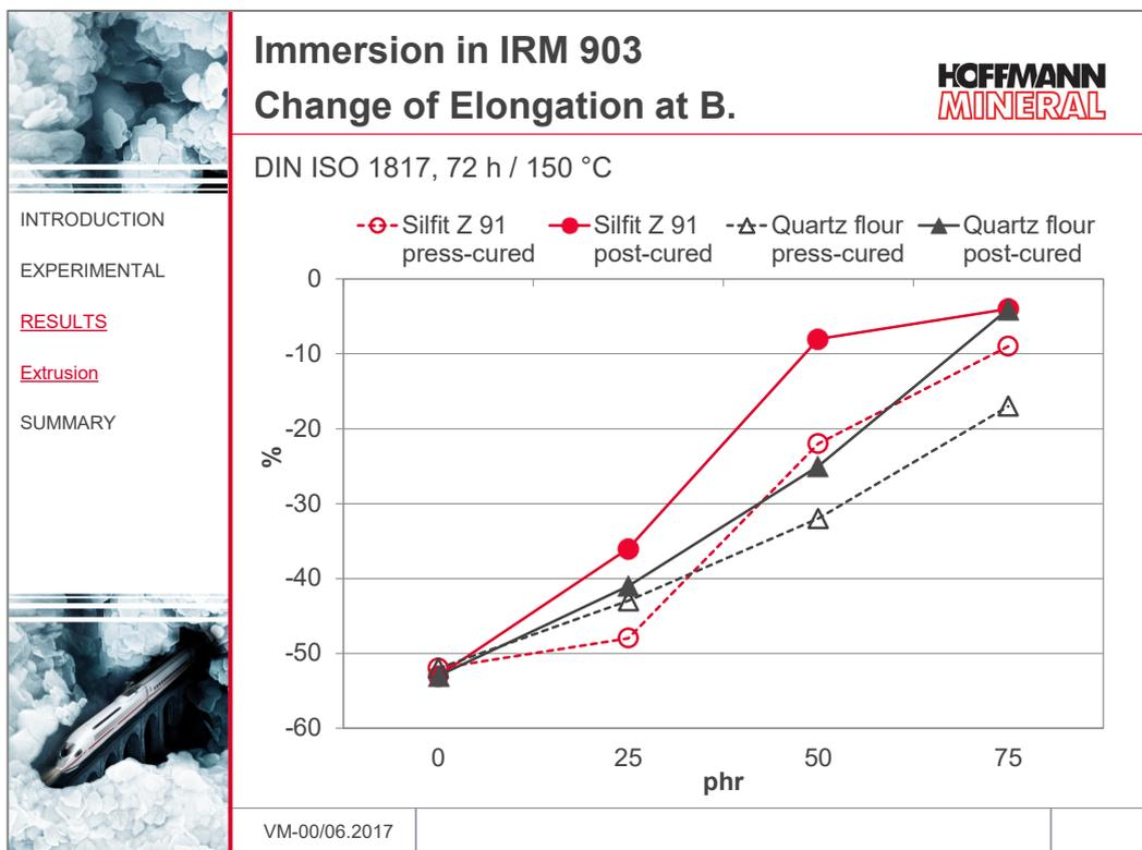
More favorable levels with the post-cured compounds containing Silfit Z 91 also result at loadings of 25 and 50 phr with respect to the elongation at break. In compounds with still higher loadings, no differences can any longer be observed between both fillers.
