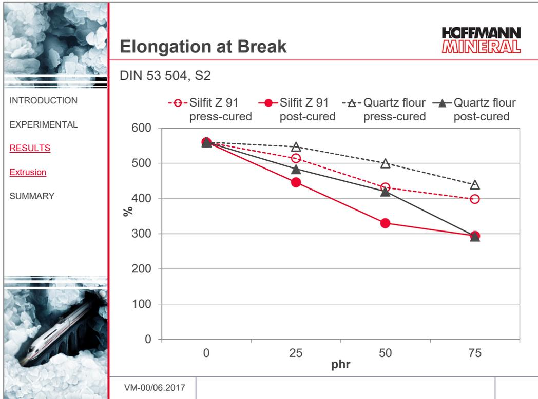
The post-cure gives rise to a decline of the elongation at break of the filler loaded compounds by 100 % (in absolute figures). With a loading of 25 resp. 75 phr, the difference between Silfit Z 91 and the quartz flour is not quite as pronounced as with 50 phr.
