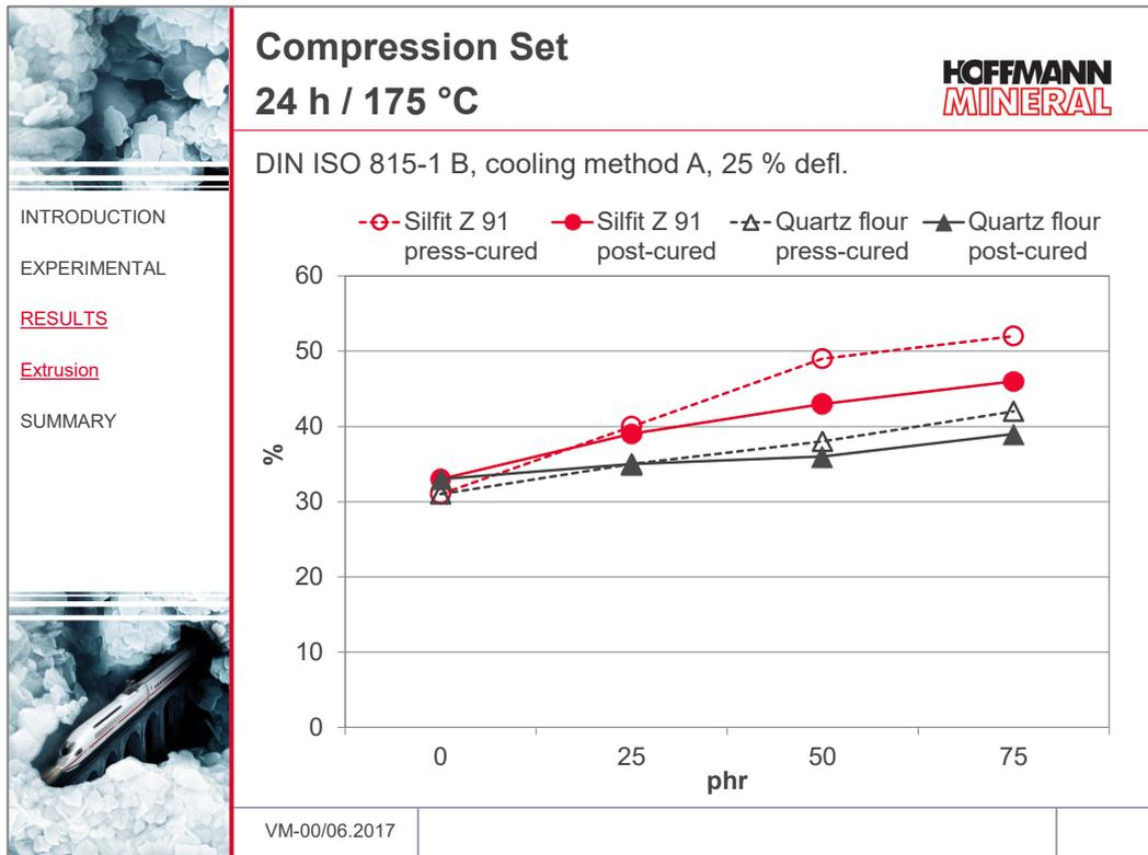
Through post-curing, the compression set of the compounds loaded with Silfit Z 91 can be decreased to a level which comes close to the quartz flour.
