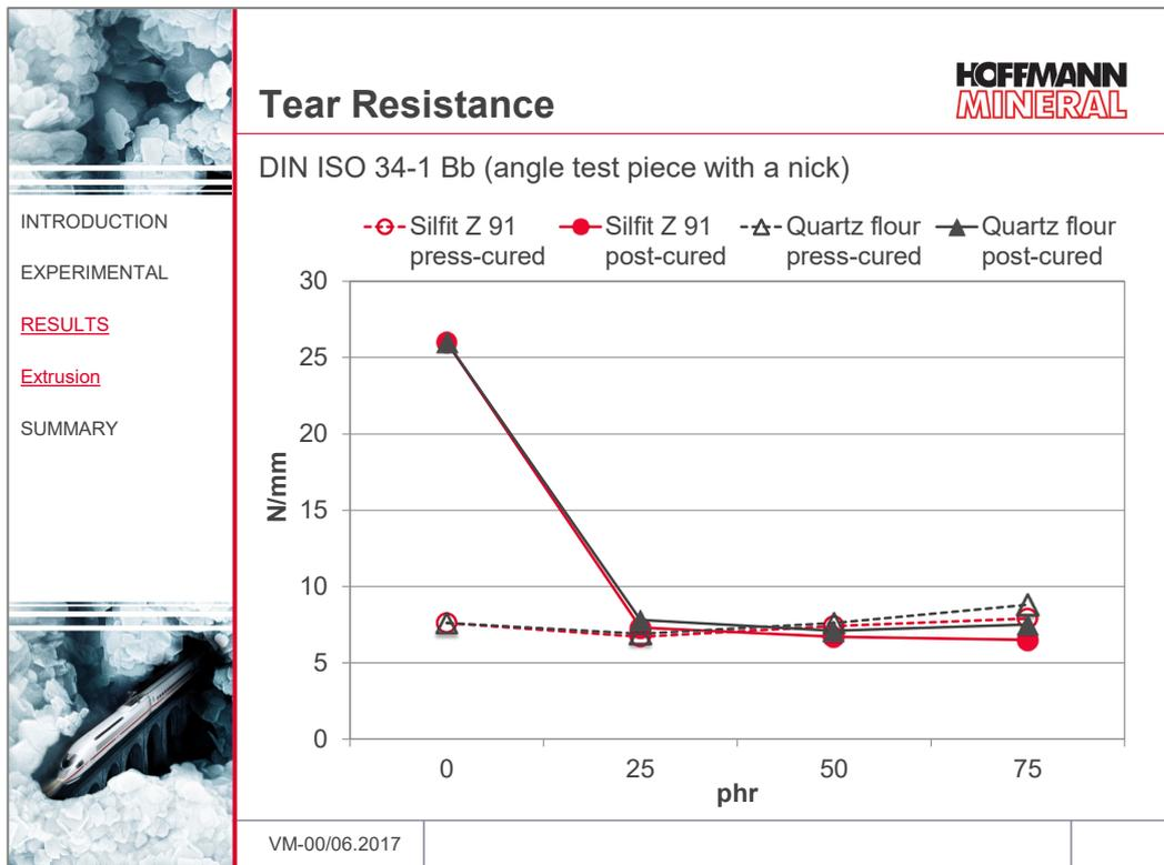
In the post-cured compounds, the addition of 25 phr filler already causes a marked drop of the tear resistance – and this irrespective of the type of filler used. With further increased loadings, no further change in the tear resistance level can be observed and there is no difference either between Silfit Z 91 and the quartz flour.
