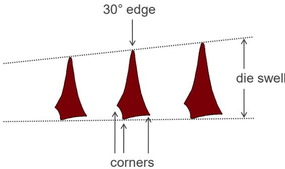
The diagram illustrates the Garvey profile with three red extruded shapes. A horizontal dashed line represents the die exit. The top of the shapes is higher, labeled 'die swell'. The top edge is angled, labeled '30° edge'. The bottom corners are rounded, labeled 'corners'.
