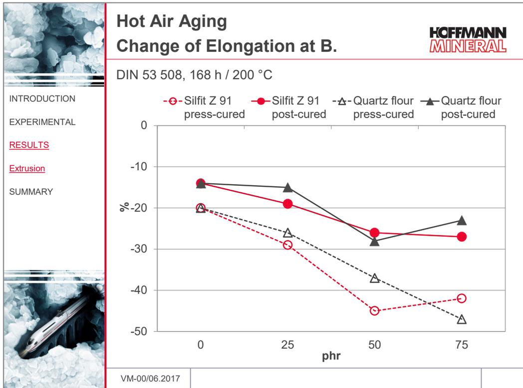
Between the two fillers, no significant differences can be found with respect to the aging in hot air (168 h / 200 °C). This is here illustrated by the changes in elongation at break. A post-cure leads to smaller changes in elongation both with Silfit Z 91 and with quartz flour.
