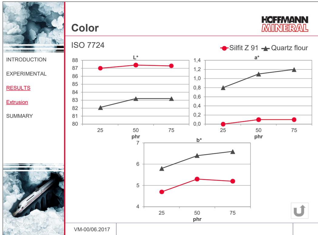
Compounds filled with Silfit Z 91 are distinctly brighter compared with quartz flour loading, as confirmed by the L\* values in the diagram. While the a\* values with Silfit Z 91 doubtless are found in the neutral region, the b\* values are clearly oriented towards a shade of blue. The result is a higher color neutrality of the compounds loaded with Silfit Z 91 in comparison with the samples with quartz flour.
