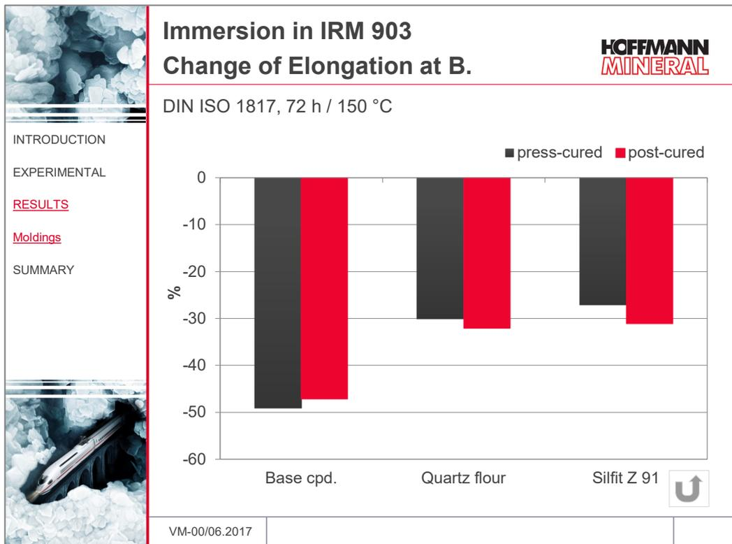
In this graph, the change of elongation at break during immersion in reference oil IRM 903 (72 h / 150 °C) demonstrates, to what extent the resistance can be improved by the addition of fillers. Silfit Z 91 and the quartz flour show comparable effects – and this before and after post-curing.
