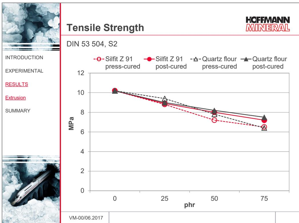
The increasing loading of fillers leads to a decline of the tensile strength of the base compound. Before post-curing, the compounds show small differences only at medium loading, while after post-cure no deviations are observed between Silfit Z 91 and the quartz flour.
